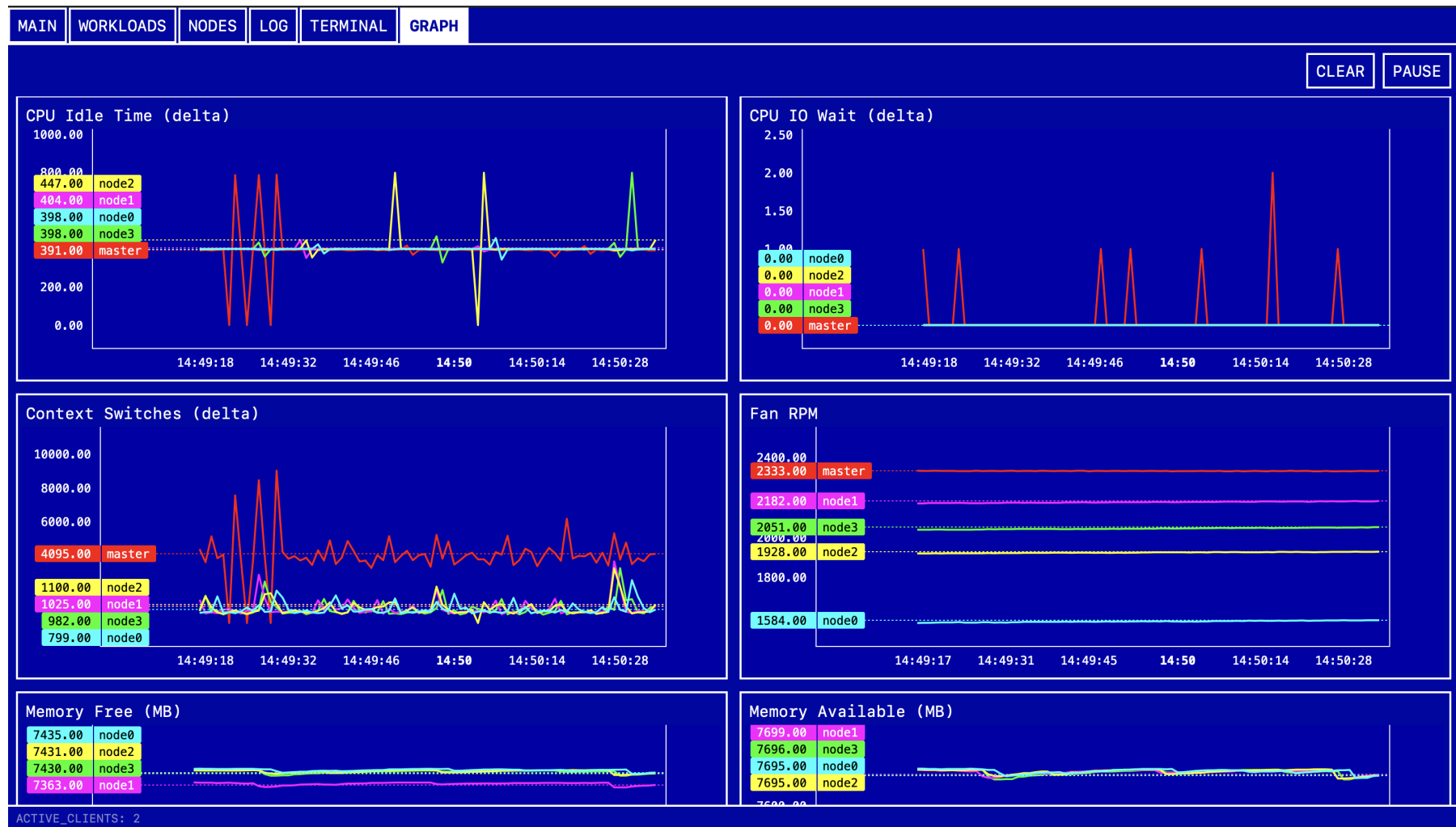
Figure A.10: The GRAPH tab, showing CPU idle time, I/O wait, context switches and fan RPM metrics.
