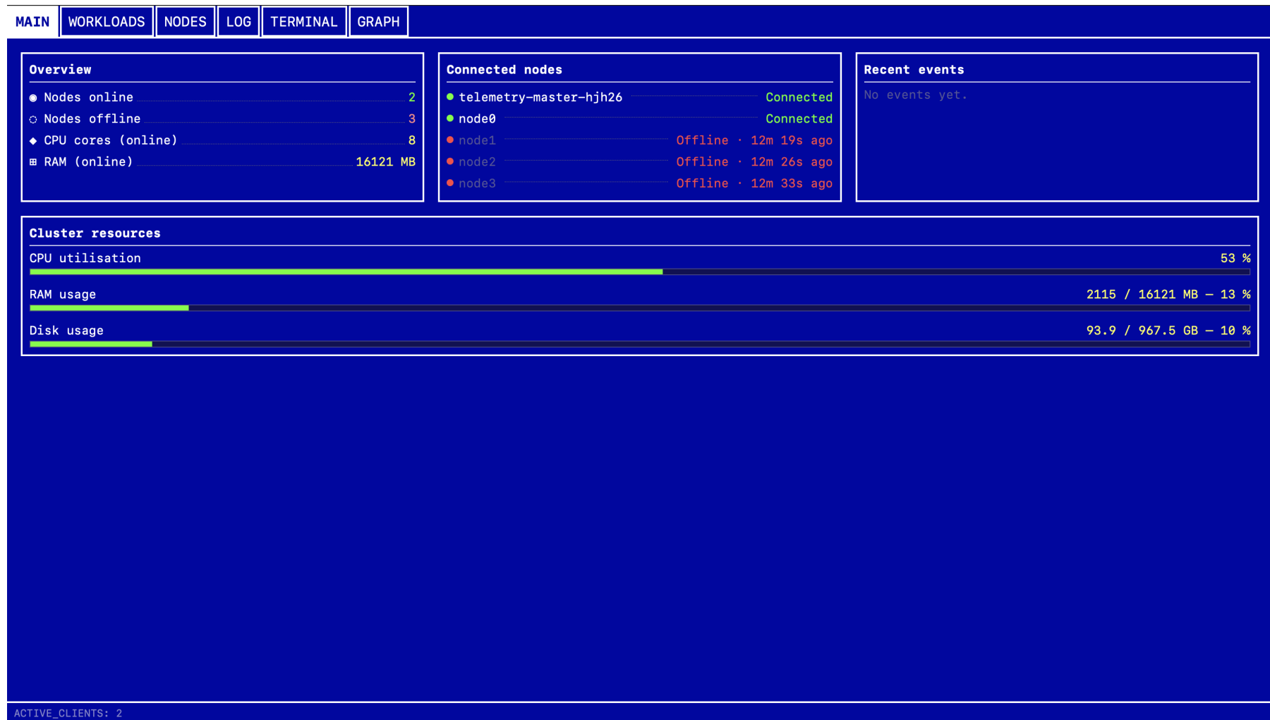
Figure A.2: The MAIN tab after three workers have gone offline. Offline nodes remain visible in the Connected nodes panel, annotated with the time since the last received report.
