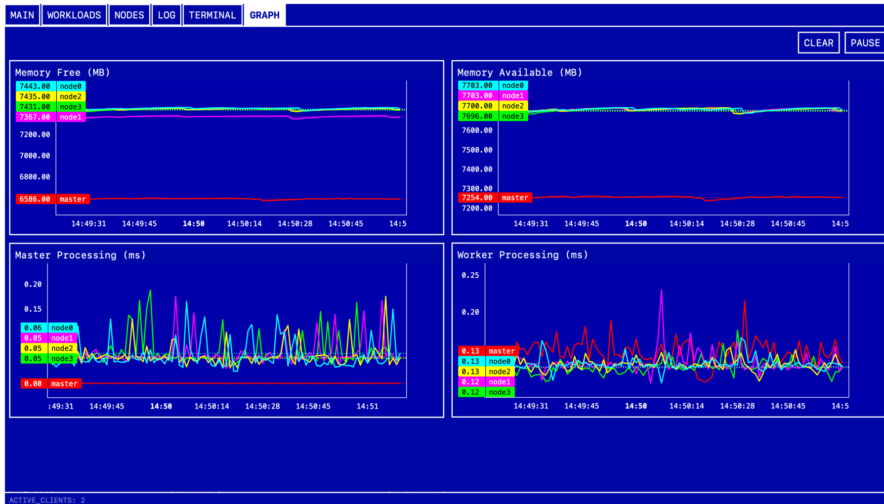
Figure A.11: The GRAPH tab, showing free and available memory on each node together with the worker and master processing latencies introduced by the telemetry pipeline.
