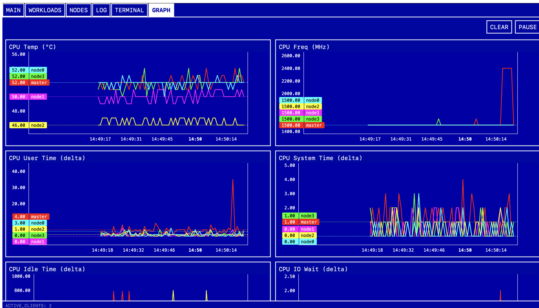
Figure A.9: The GRAPH tab, showing CPU temperature, current frequency, and the user and system time counters as live time-series across the cluster.
