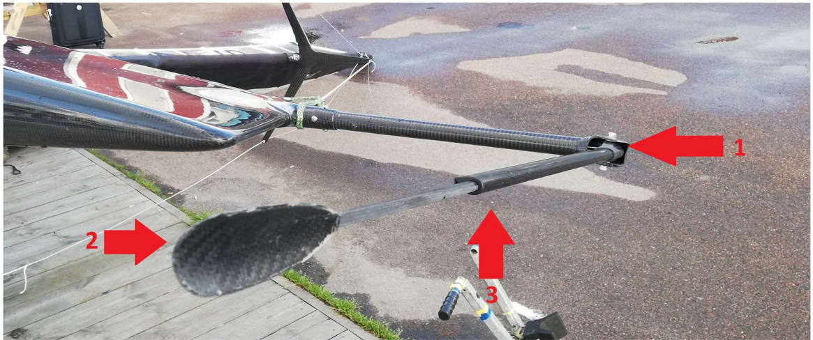
Figure 5.2 The Mach2 wand solution (Boman, 2019).
