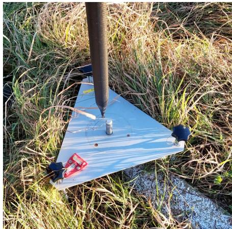
**Figure 4.17:** Measurements were taken on a screw hole of a triangular metal plate.
