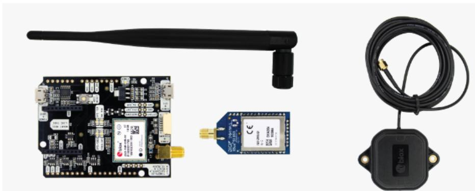
**Figure 3.1:** The u-blox simpleRTK2B test kit contains two identical sets of components in the above figure [40]. Starting from the top, clockwise: radio antenna, GNSS antenna, LR radio module, u-blox ZED-F9P receiver board.
