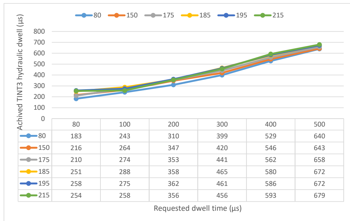
Figure 8.19 - Requested TINT3 hydraulic dwell vs Achieved TINT3 dwell at different rail pressures (80, 150, 175, 185, 195 & 215 MPa) for pilot quantities doubled
