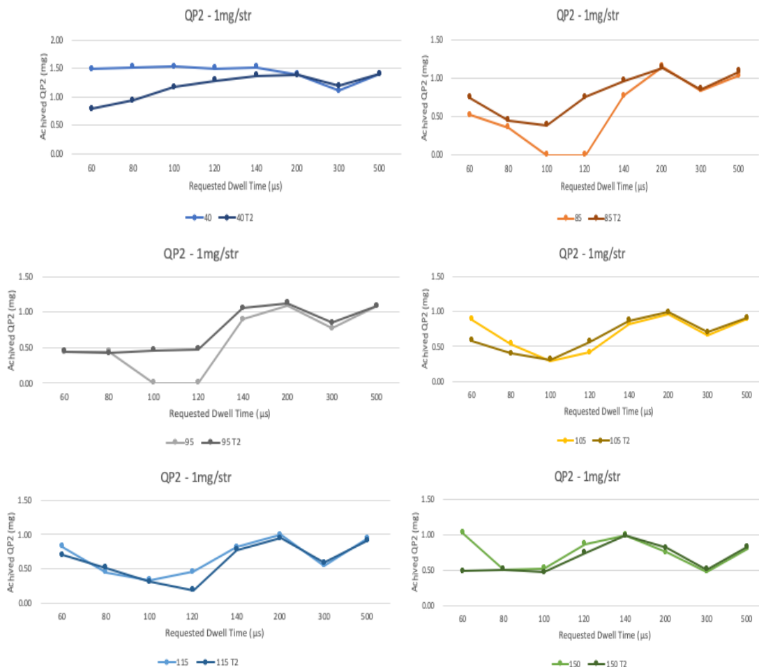
Figure 4.27 - Achieved QP2 fuel quantity vs Requested TINT2 separation at different rail pressures (40, 85, 95, 105, 115, 150 MPa)
