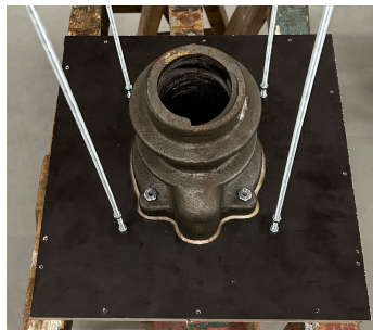
Figure 3.11: Mould side where the anchor system and metallic rods were mounted.
