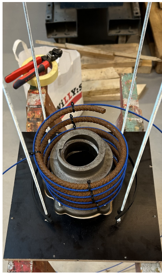
(a) Attachment of fibre optics on the anchorage reinforcement.
