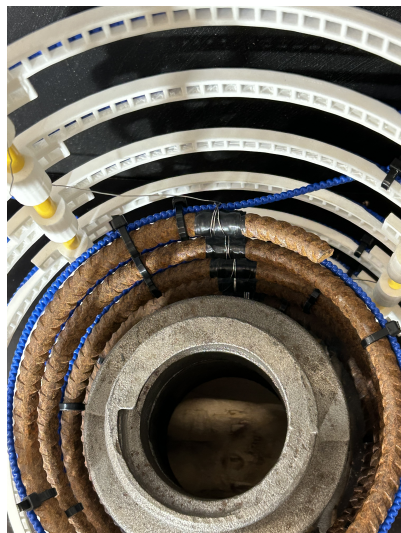
(a) Winding of Kanthal wire around the anchorage reinforcement.
