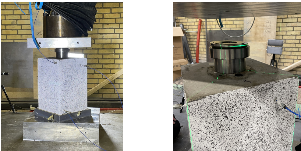
Figure 4.6: Concentric load setup and positioning of specimen.
