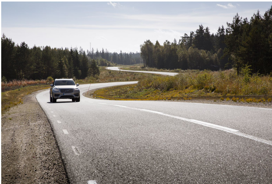
Figure 3.2: Large amplitude road for primary ride evaluation.
