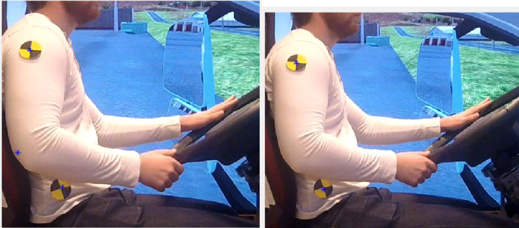
Figure 13: Example of one mark being occluded by the arm of the driver. In the left image, the point tracker is allowed to continue tracking when the mark is occluded, resulting in the blue star on the elbow. In the right image the point tracker has been re-initialized to only track the two visible marks.
