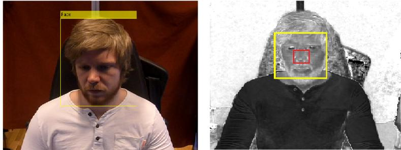
Figure 28: In the first frames of each video, the drivers face was detected and within this region the nose was detected (right). A Camshift tracker applied to this region in the saturation channel of the HSV color space was used to track a bounding box surrounding the drivers face.
