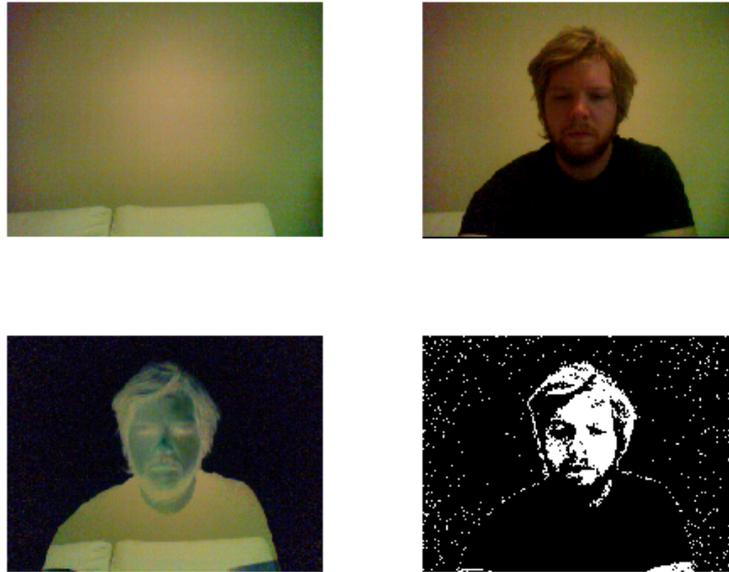
Figure 27: An example of motion-based binarization. Background image (top left), current frame (top right), difference of current frame and background frame (bottom left) and binary image of thresholded difference (bottom right).
