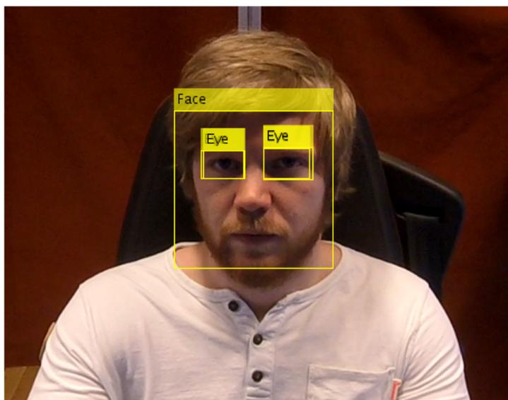
Figure 33: The drivers eyes detected using the extension of the Viola-Jones algorithm by Yu Shiqi.
