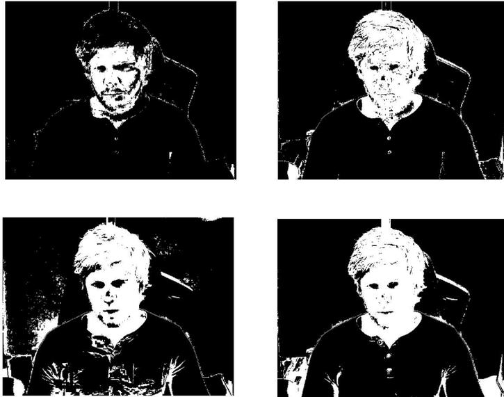
Figure 32: Several methods were tried for color-based binarization. Thresholding in RGB color space (top left), HSV (top right), YCbCr (bottom left) and histogram based likelihood thresholding in RGB (bottom right).
