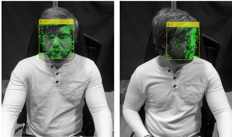
Figure 16: Driver with bounding box around face (yellow) and KLT feature points (green marks). The points are approximately normally distributed around the center of the image when the driver looks straight ahead (left), but when the driver turns his head (right) the mean and standard deviation are greatly changed.
