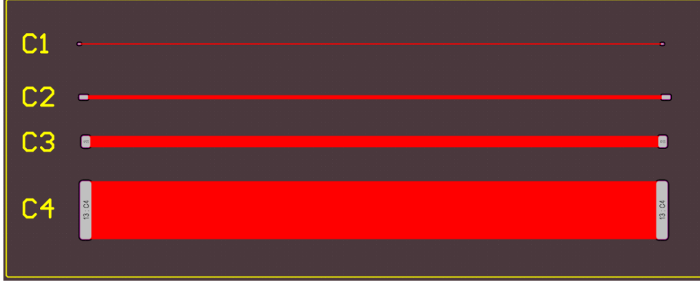
Figure 3.11: Structure C showing conductors with increasing width from C1 to C4.
