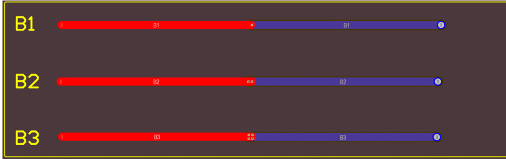
Figure 3.10: Structure B showing via arrays with increasing number of vias for current transition between layers.
