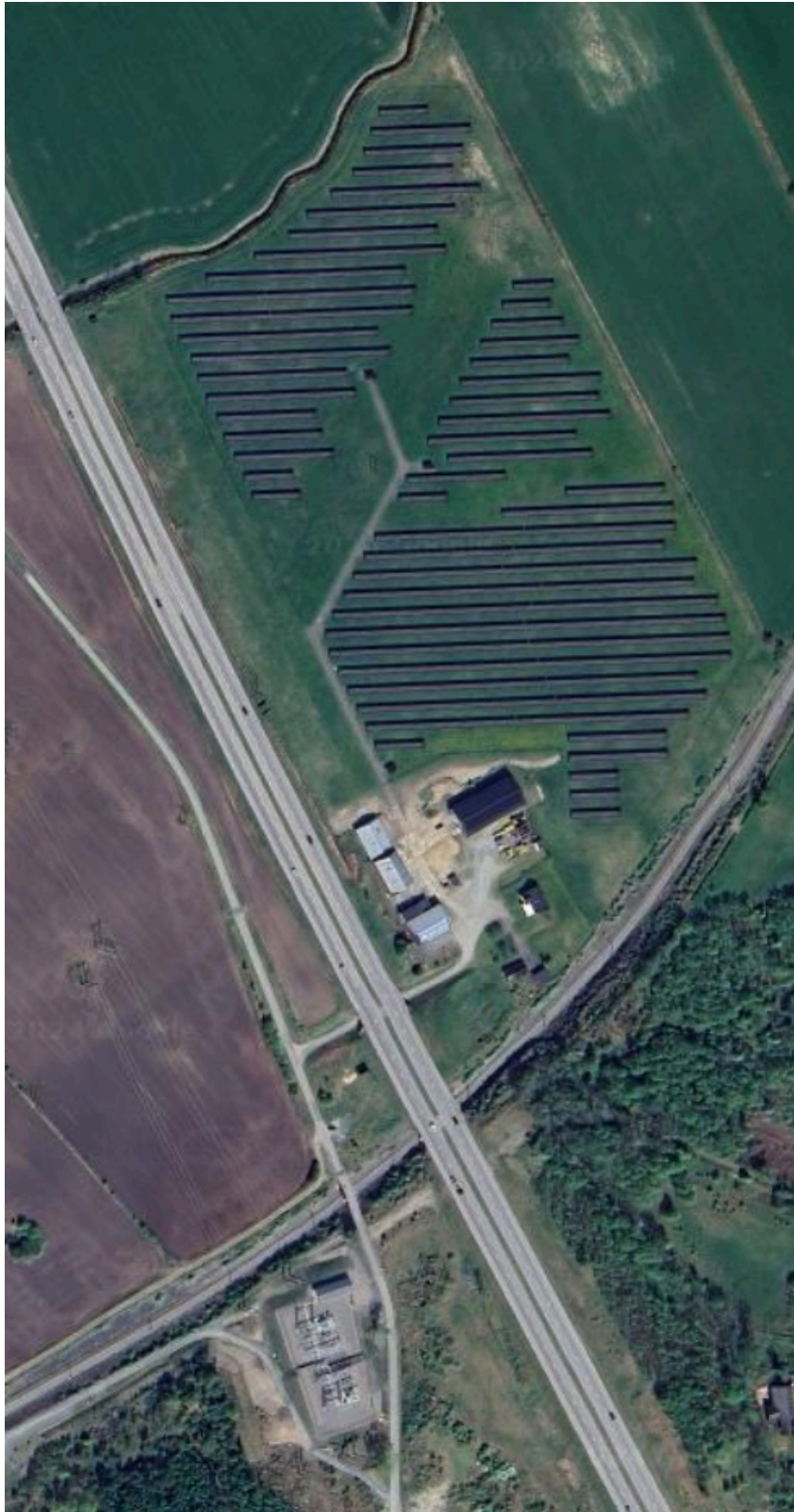
Figure I.II PV park Varberg Norra and supposed connection to new substation less than 500 m away (C google Earth). Corresponding to category “new infrastructure”.
