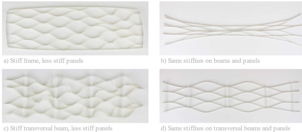
Figure 6.5 Experimental models of actively bent cardboard and paper strips.
