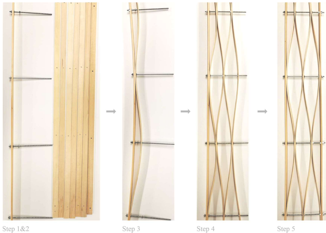
Figure 6.8 Diagram of the assembly method of the concept model.
