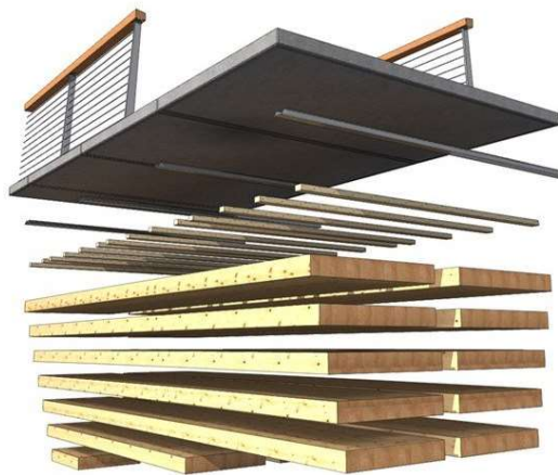
Figure 3.4 Exploded view drawing of the Neckartenzlingen Pedestrian Bridge (Ingenieurbüro Miebach, 2017). Illustration created by Ingenieurbüro Miebach. Used with permission.
