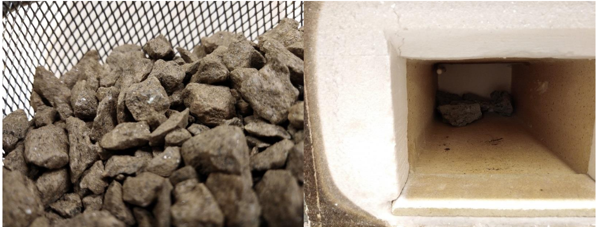
Figure 2. The smaller fragments (left hand side) required 4 hours to achieve satisfactory dehydration of the calcium silicate hydrate. Whilst the larger chunks (right hand side) needing 7 hours for it.
