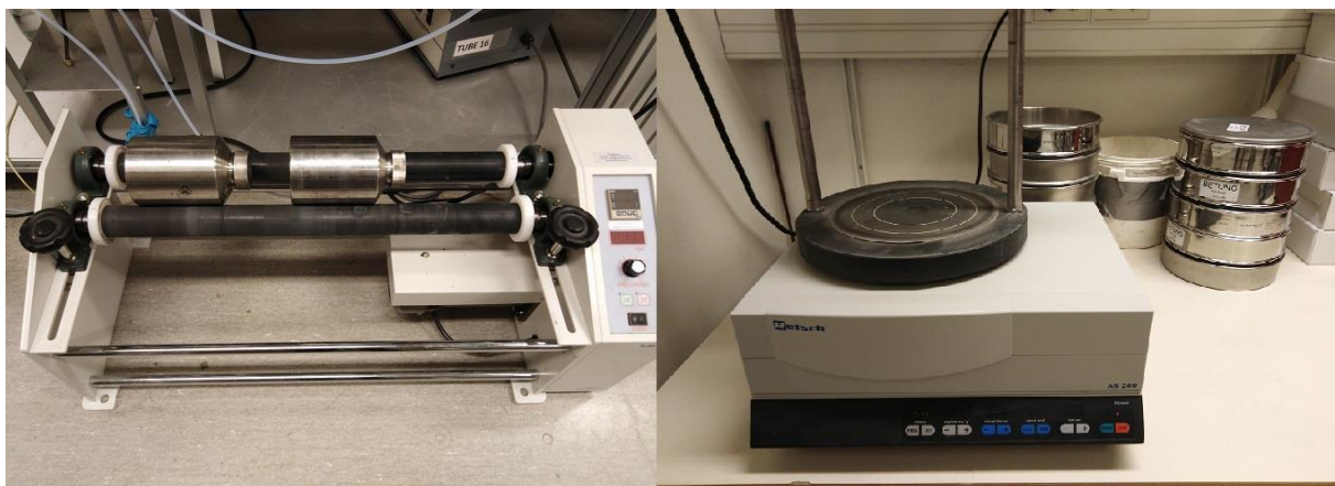
Figure 3. The ball mill with the steel containers that was used on the left-hand side. On the right-hand side, the sieve with the varying sizes of filters stacked to the side of it.
