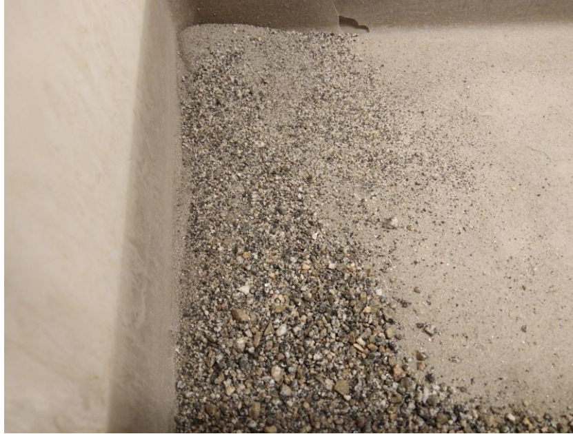
Figure 5. The process of creating pulverized recycled aggregates. The larger particles were crushed with a steel hammer until reaching a certain size and were then sieved. This process was repeat several times.
