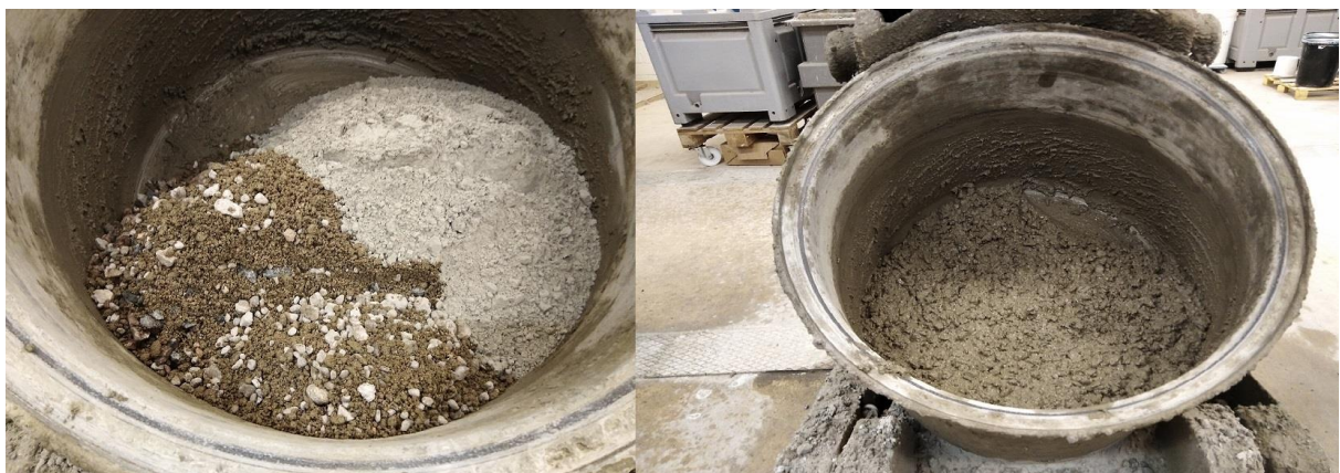
Figure 6. The process of making one of the concrete batches.
