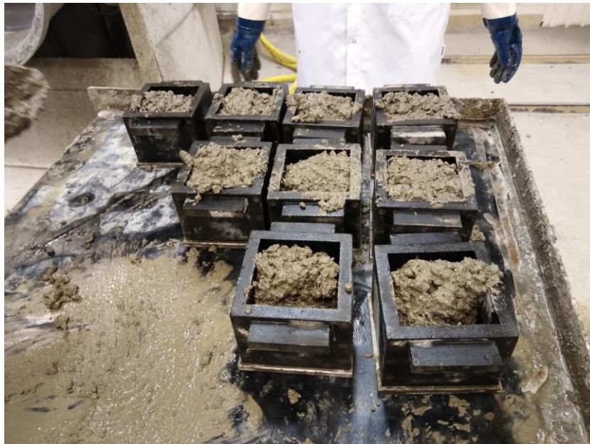
Figure 8. The concrete test cubes before they have been smoothed out using the shake board.
