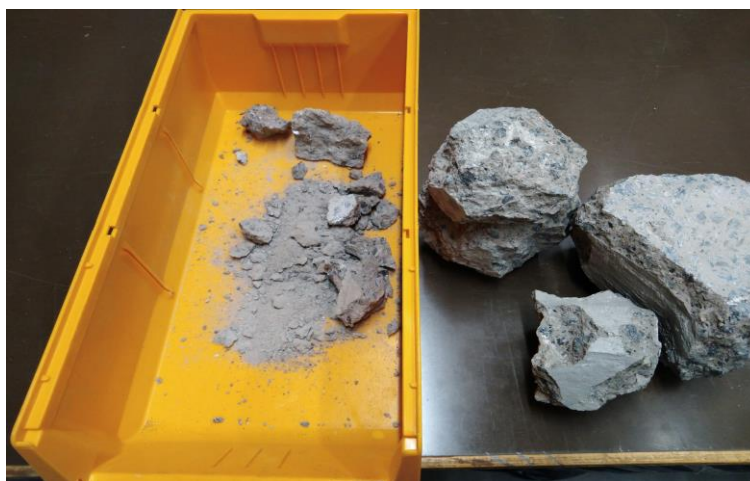
Figure 1. The supplied concrete the rough size it was broken down to in the first step.
