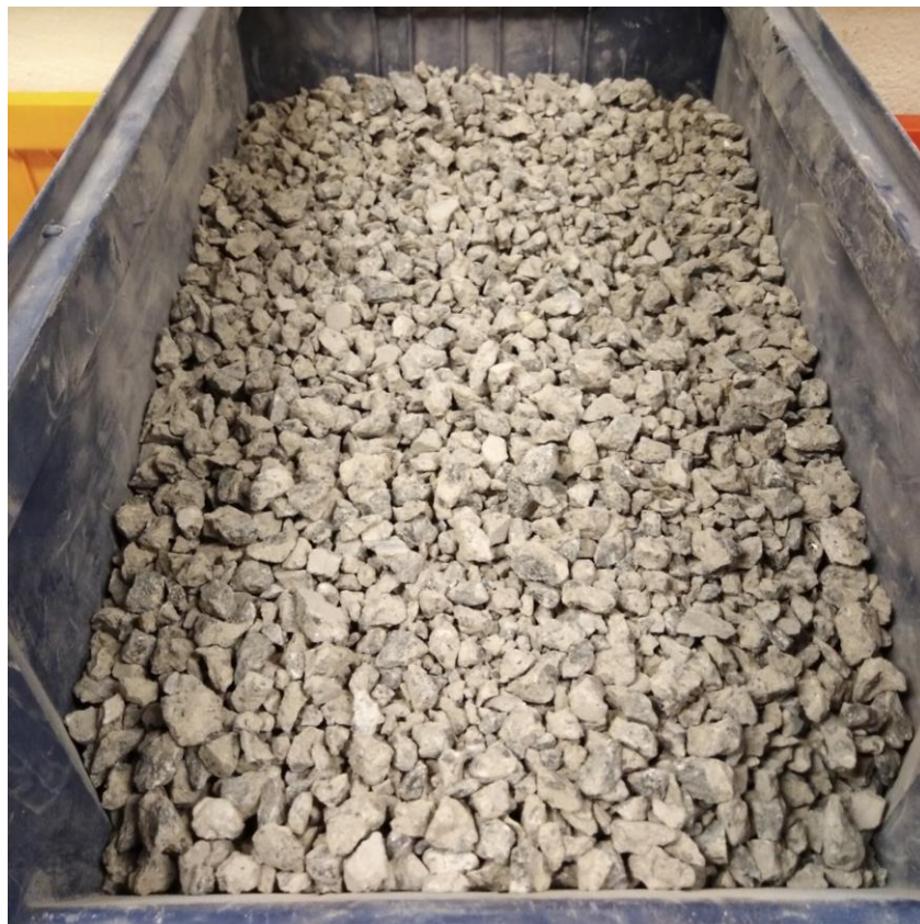
Figure 4. The final RCA, fraction size 4-16 mm, after washing with water.
