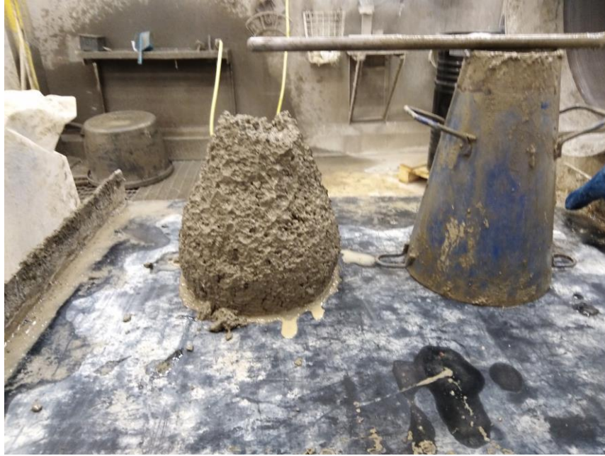
Figure 7. The slump flow test measures the height difference from the top of the cylinder to the top of the concrete after a predetermined time interval.
