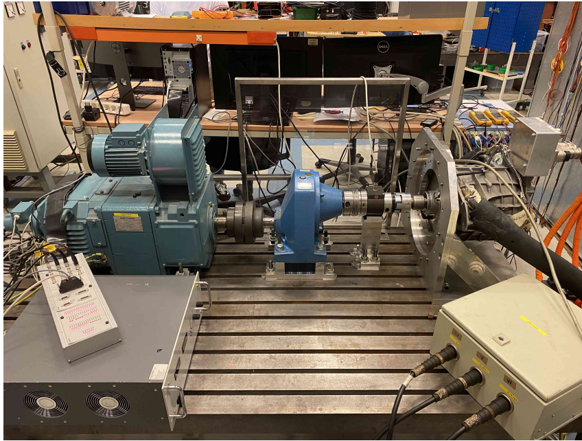
Figure 4.8: A picture showing the connection made between the large machine and the DC machine.
