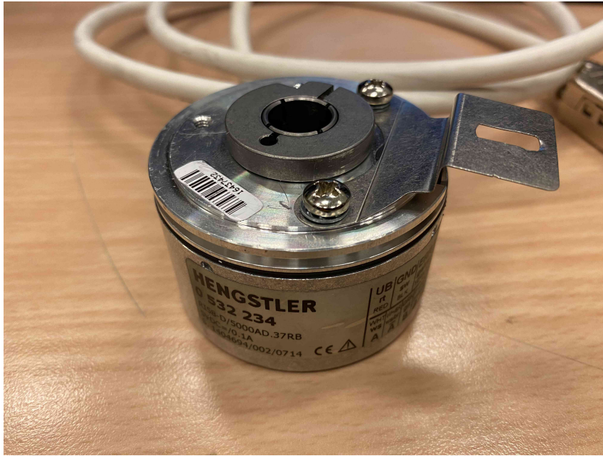
Figure 4.5: The incremental encoder giving 5000 pulses per revolution used for operating the small machine.
