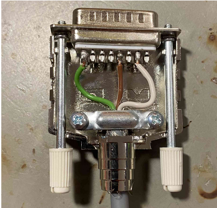
Figure 4.6: Wires from the encoder soldered onto a digital I/O connector. This picture was taken during the first attempt of measuring the speed in dSPACE. However when the frequency block in dSPACE was implemented, the white and green cables which contains pulse train A and ground was soldered to another digital I/O connector with 37 pins to be processed in dSPACE.
