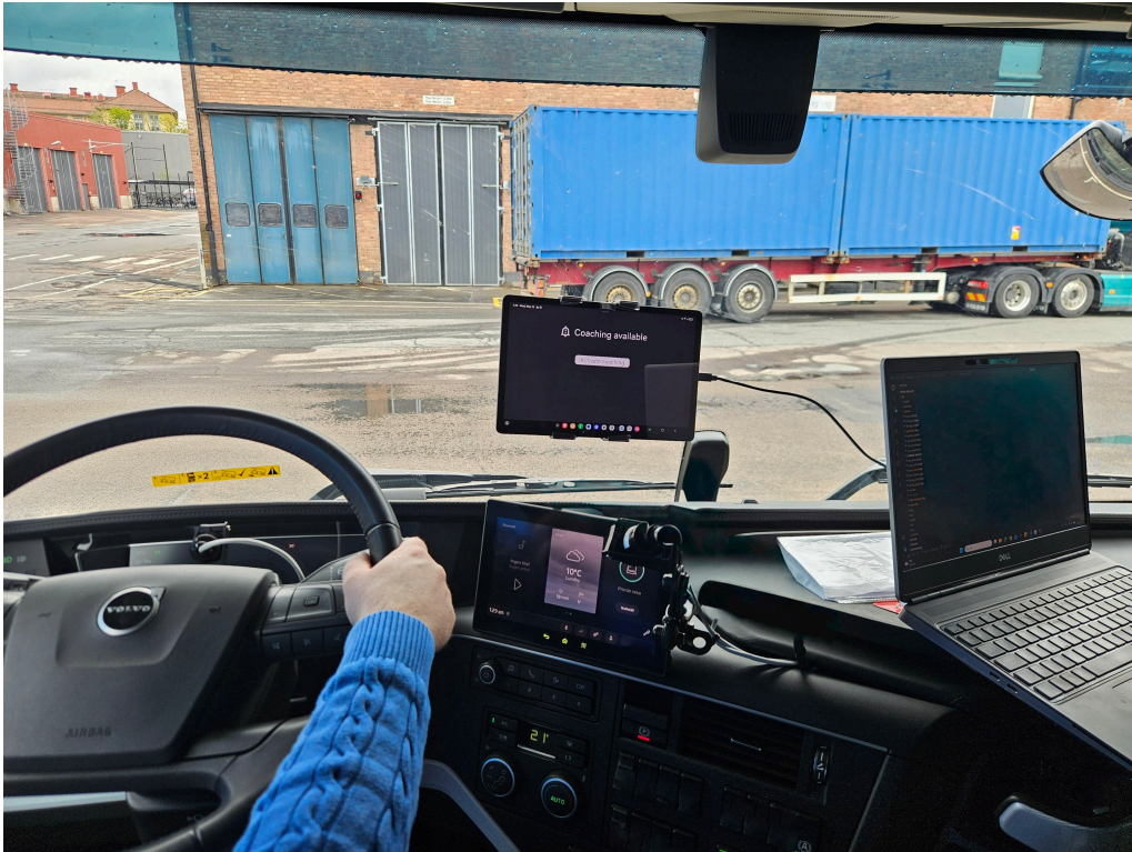
Figure 5.5: Example of the prototype evaluation setup inside the truck cabin. Parts of the image have been edited using generative AI tools to preserve confidentiality.
