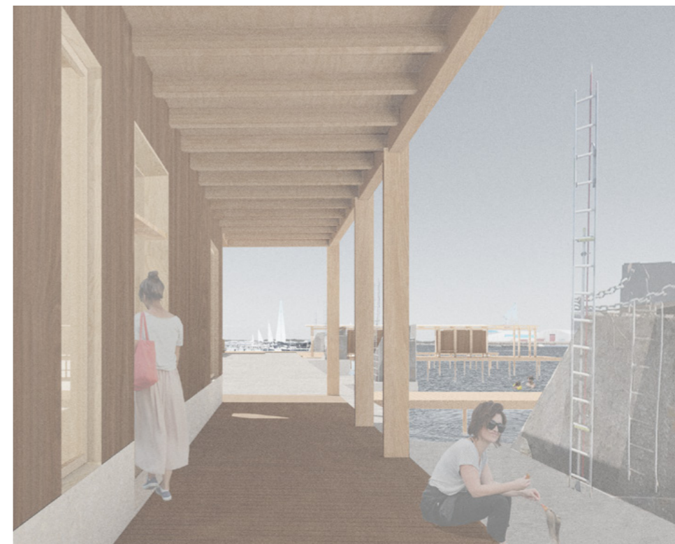
Fig 35. The large roof and the high concrete base protect the facade from the west coast's harsh climate, as a response to design principle 5.c.
