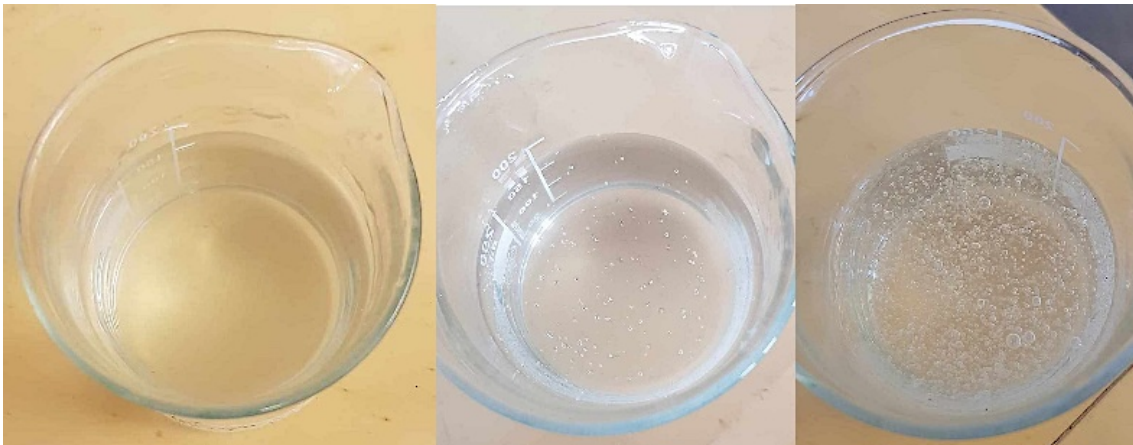
Figure 4.3: Phantom Appearance of Natrosol 250 HHX at Various Concentrations: Left: 3wt% to Right: 4wt%
