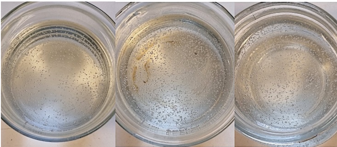
Figure 4.4: Phantom Appearance of Natrosol 250 HHX at Various Mixing Velocities: Left: Phantom 1 to Right: Phantom 3
