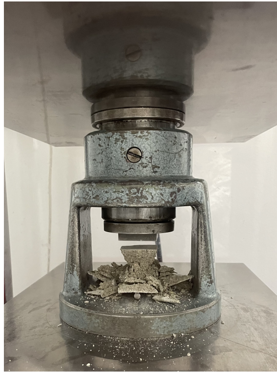
Figure A.1: Broken, F50 mortar
