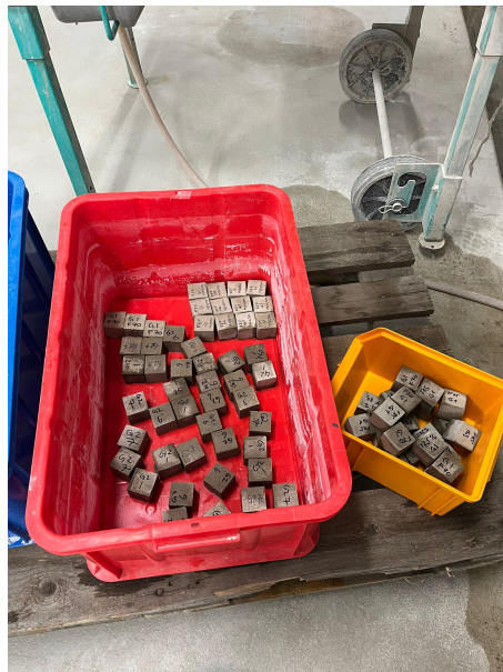
Figure 3.11: Samples stored in water-filled containers
