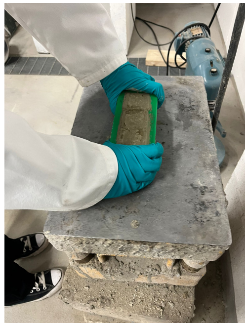
Figure 3.8: Vibration of the mixture
