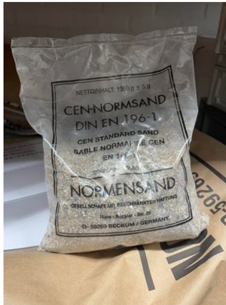
Figure 3.1: Specified aggregates, Normsand DIN EN 96-1
