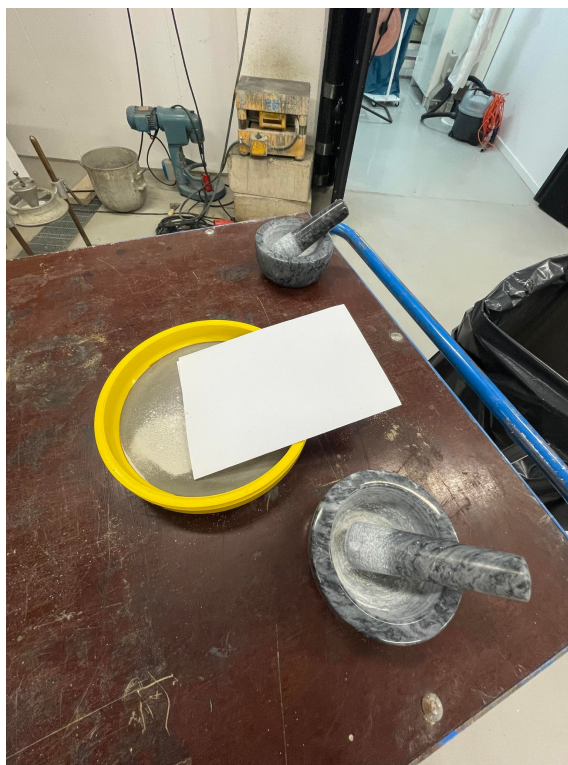
Figure 3.14: Mortel and sieve for crushing samples
