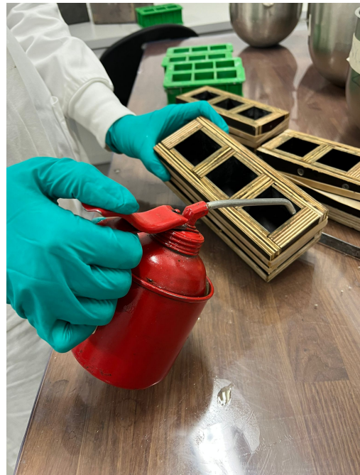
Figure 3.6: Distributing the oil in the molds
