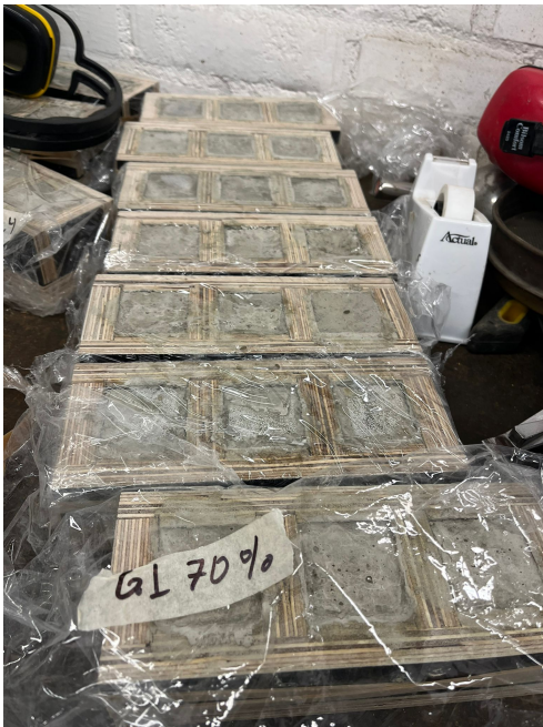
Figure 3.9: Plastic wrapped molds
