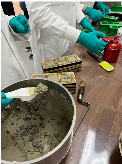
Figure 3.7: The molds filled with the mixture
