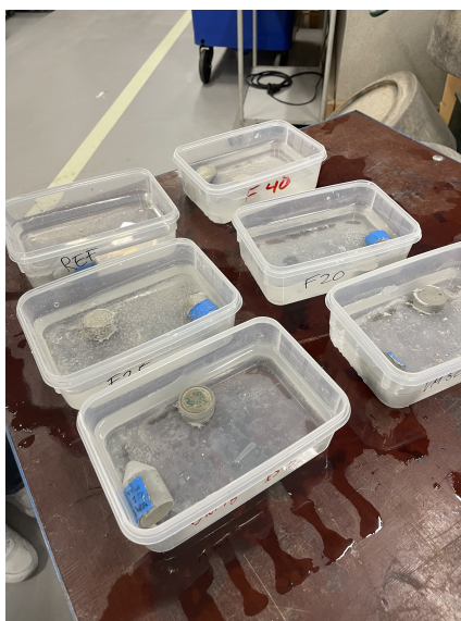
Figure 3.13: Sawed paste samples curing in water
