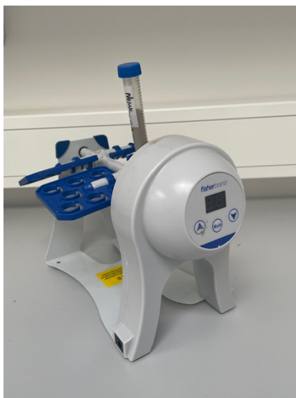
Figure 3.12: Rotator used for rotating the pastes
