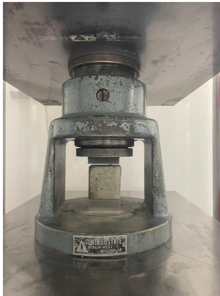
Figure 2.1: Compressive strength test machine on a mortar
