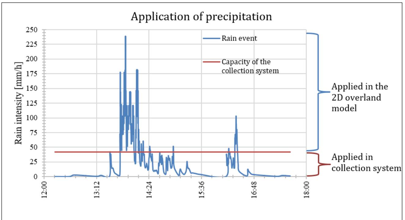
Figure 11. An example of which parts of a rain event that is applied in the 2D overland model and in the collection system, respectively.
