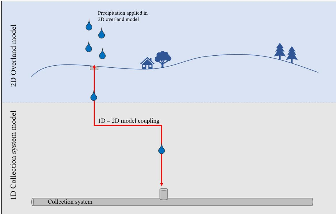
Figure 6. Illustration of precipitation applied in the 2D overland model. Illustration made by the authors.
