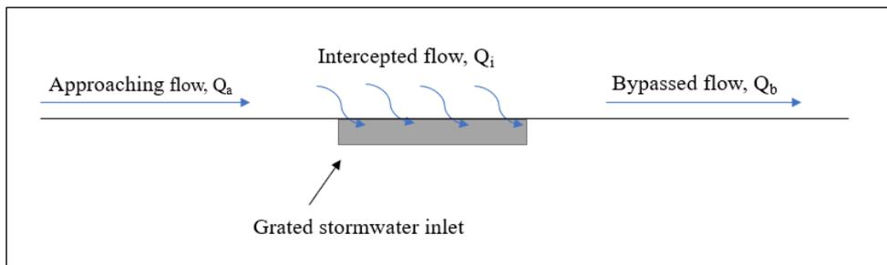
Figure 3. Illustration of the associated flows for hydraulic performance of a grated stormwater inlet. The Figure is inspired from Zaman et al. (2021) and made by the authors.
