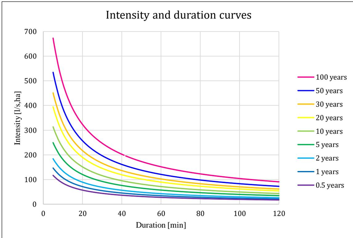
Figure 1. Intensity and duration curves calculated with Equation 2.
