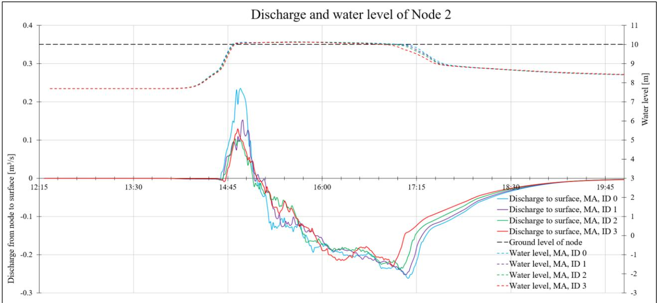
Figure 29. Discharge and water level of Node 2.
