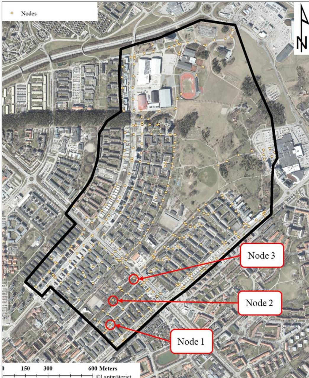
Figure 27. The three nodes analysed regarding discharge to surface and water level. Aerial photo from SCALGO Live (n.d) ©Lantmäteriet.
