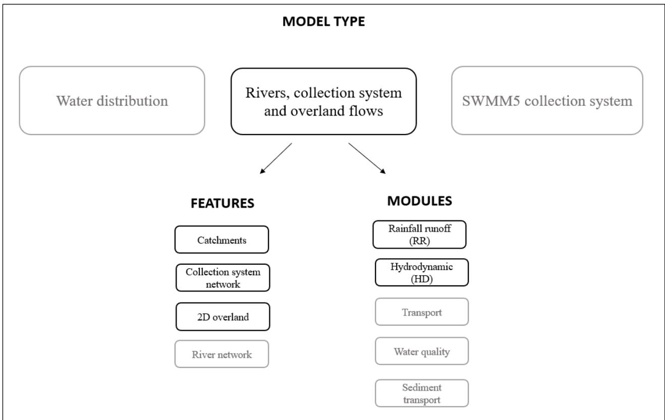
Figure 4. Conceptual scheme of features and modules associated with the model type rivers, collection system and overland flow in MIKE+. The thesis concerns boxes marked in black. Shaded boxes are not concerned in this thesis and will not be explained further.
