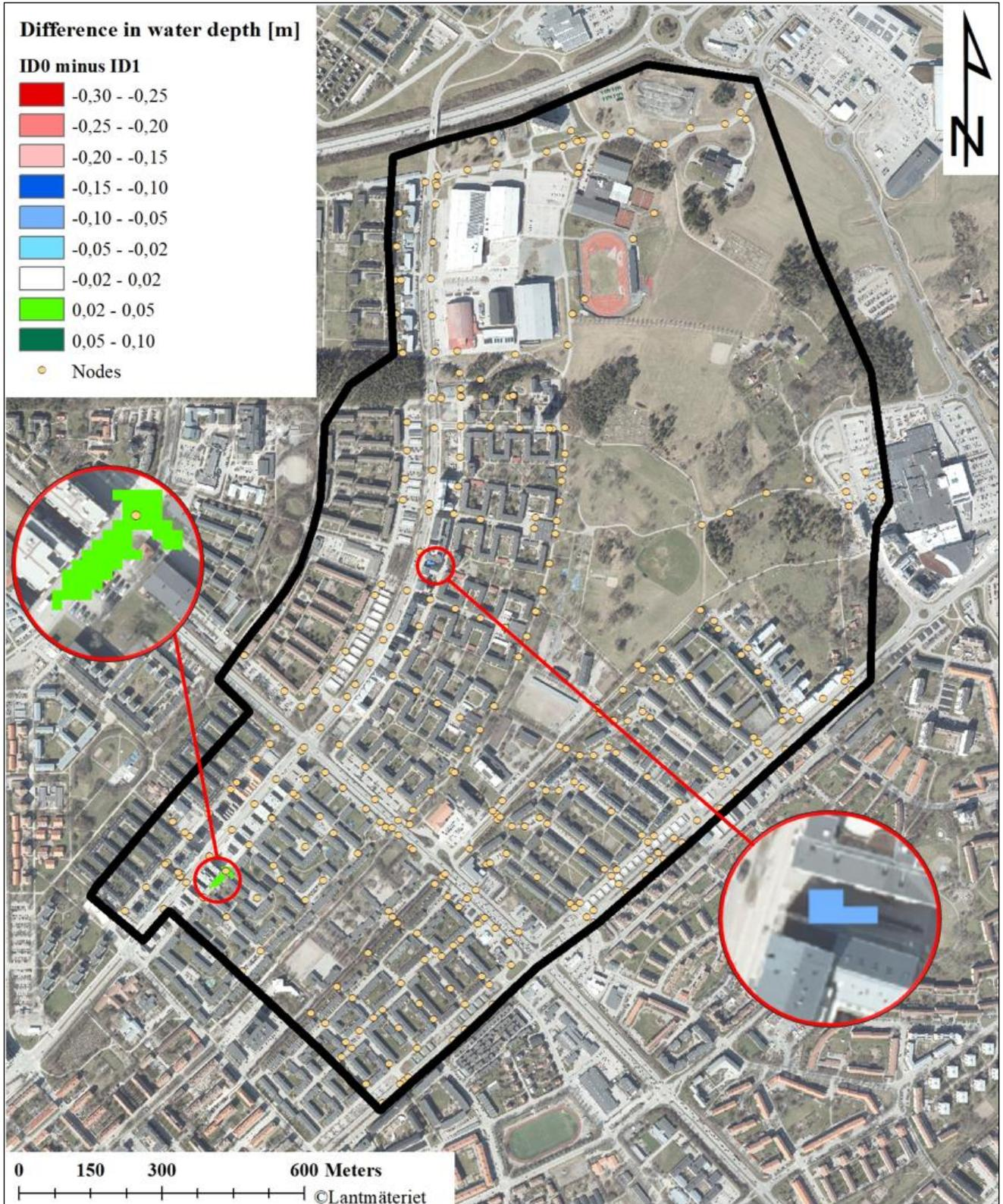
Figure 24. Difference in maximum water depth for simulation ID 0 minus simulation ID 1. Aerial photo from SCALGO Live (n.d) ©Lantmäteriet.
