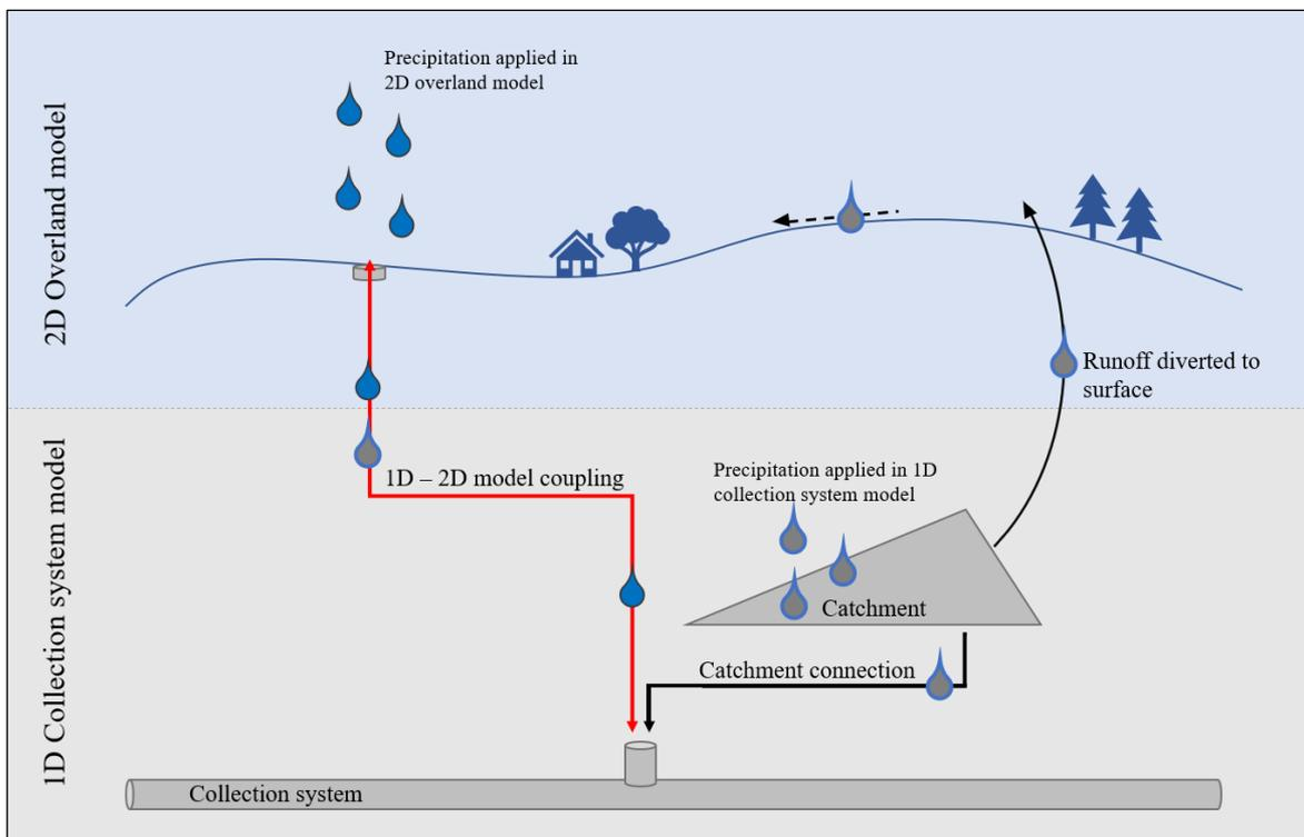
Figure 7. Illustration of precipitation applied in both in the 1D collection system model as a catchment load and in the 2D overland model. Illustration made by the authors.
