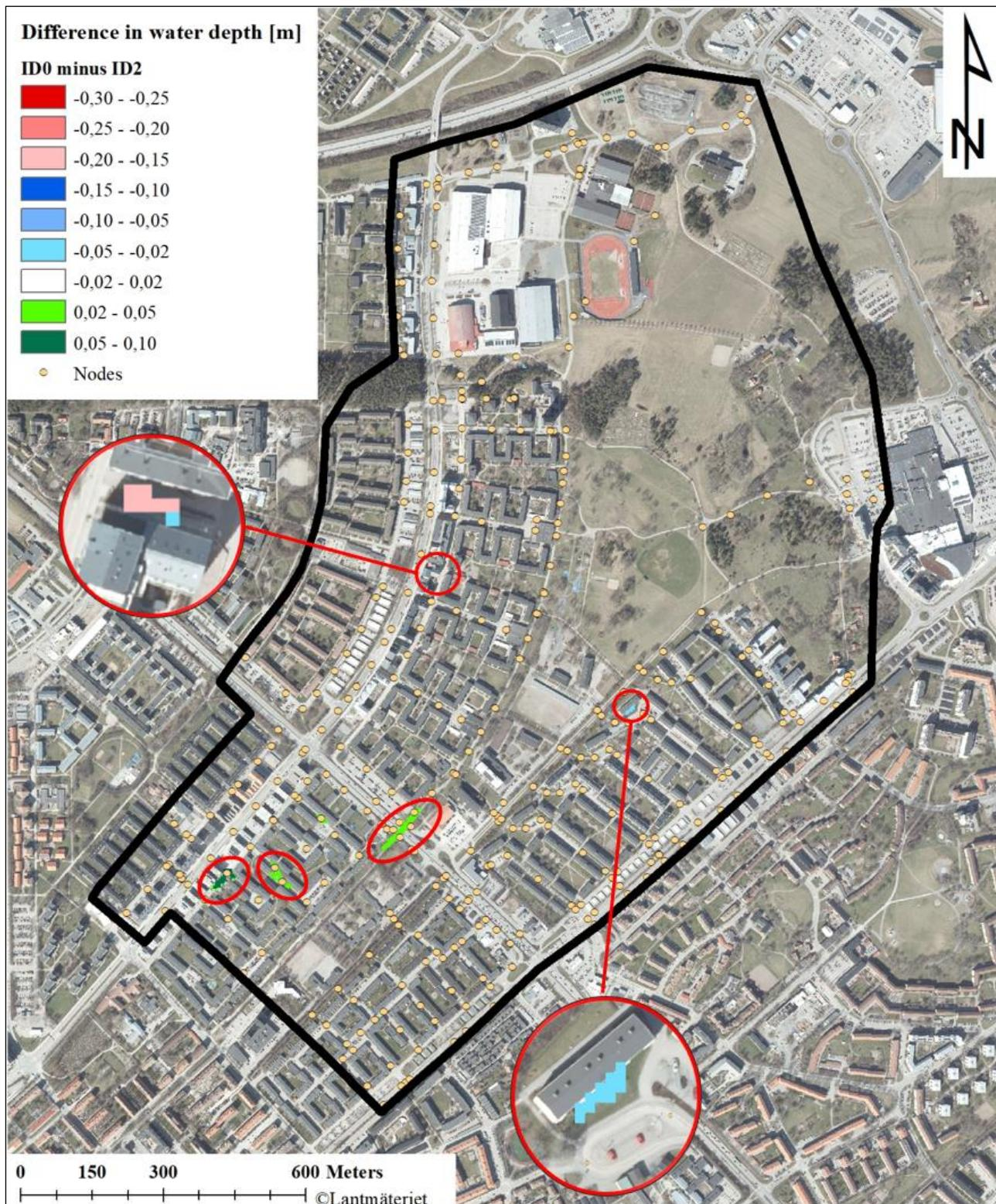
Figure 25. Difference in maximum water depth for simulation ID 0 minus simulation ID 2. Aerial photo from SCALGO Live (n.d) ©Lantmäteriet.
