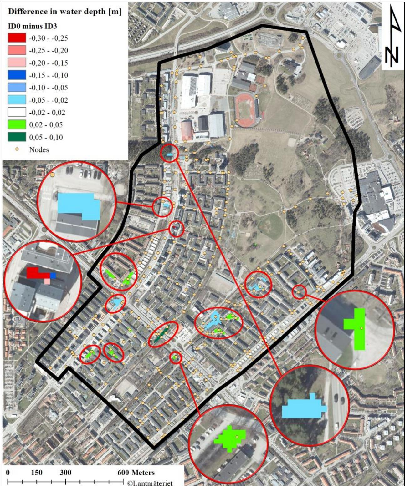
Figure 26. Difference in maximum water depth for simulation ID 0 minus simulation ID 3. Aerial photo from SCALGO Live (n.d) ©Lantmäteriet.
