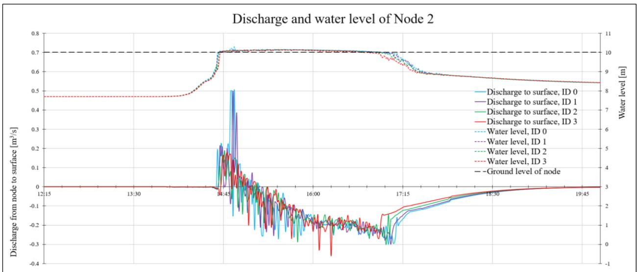
Figure B2. The figure presents the original result of discharge to surface and water level in Node 2.
