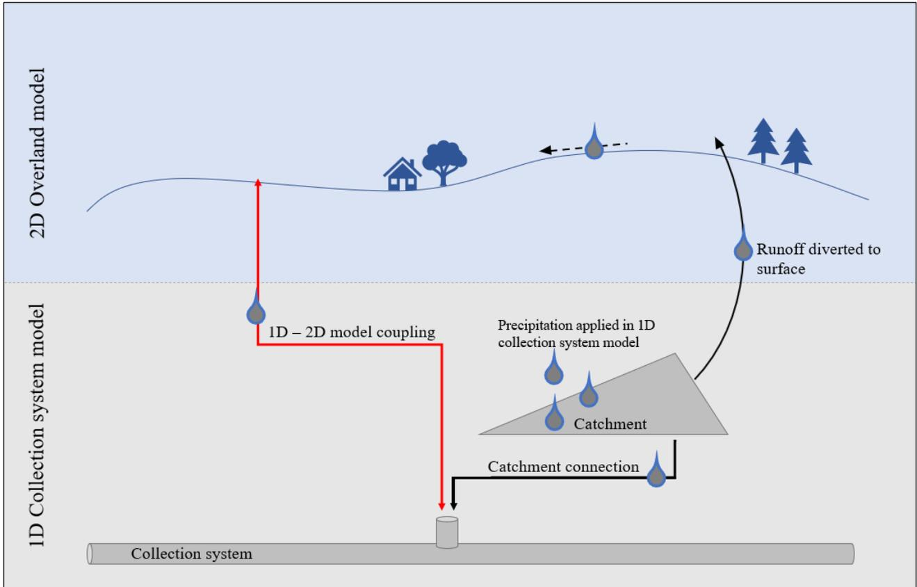
Figure 5. Illustration of precipitation applied in the 1D collection system model as a catchment load. Illustration made by the authors.
