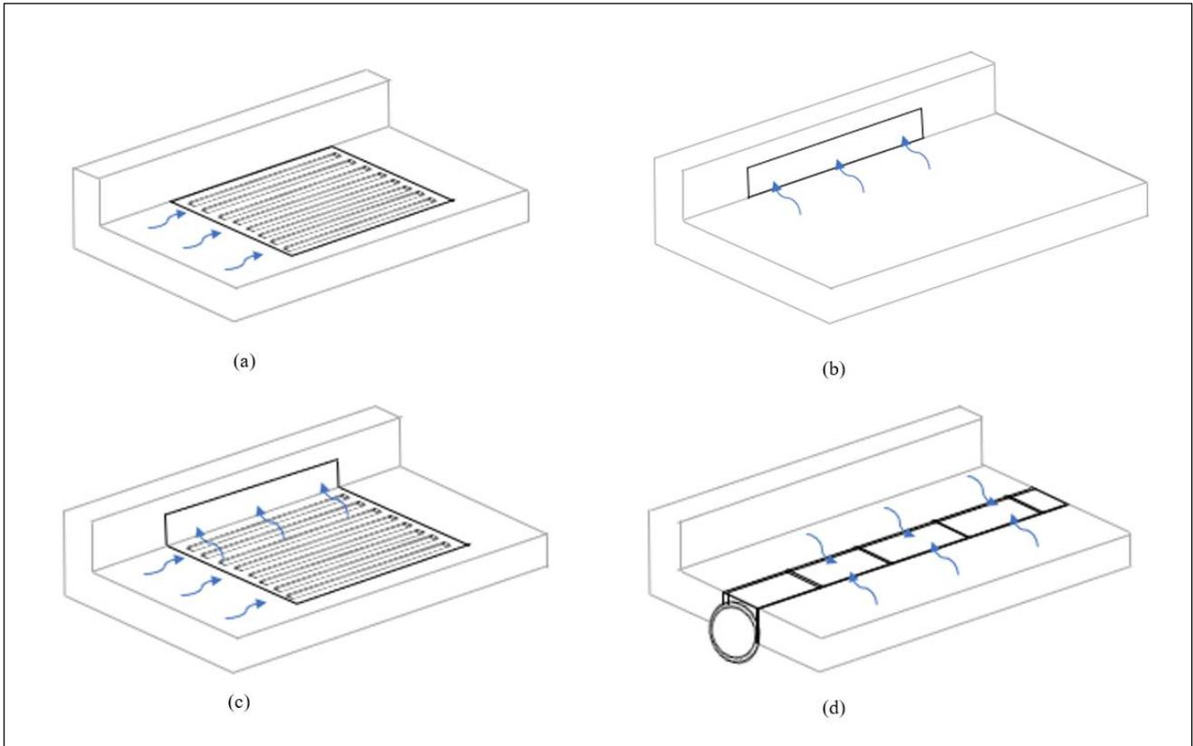
Figure 2. Illustration of stormwater inlets. (a) Grated inlet, (b) a curb inlet, (c) a combination of grate and curb, (d) and a slotted drain inlet. The illustration is inspired by UDFCD (2016) and made by the authors.
