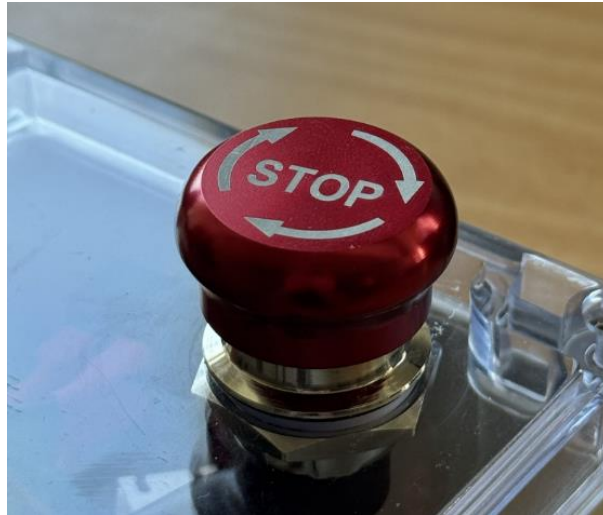
Figure 7. Emergency stop-solution for lathe controller. The emergency stop button is located on top of the application, allowing for easy access if needed. (Image by the author)
