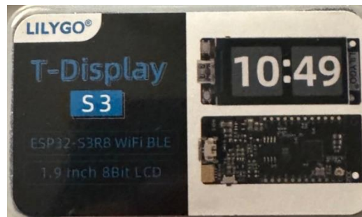
Figure 5. ESP32 and TFT display (T-Display S3) from LilyGo (image by the author).
