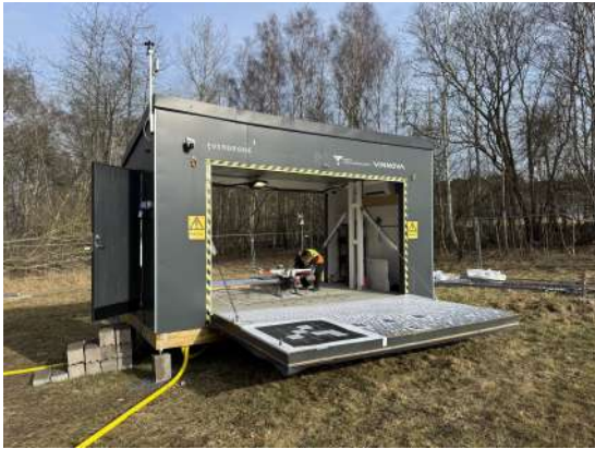
Figure 2.1: Drone hangar in Mölnådal, from which drones are automatically deployed upon identification of an emergency call requiring DEMS.
