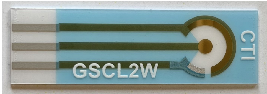
Figure 3.2: Photograph of Au-SPE used in the EG-FET system, the WE geometric area is approximately 3.14\text{mm}^2 .
