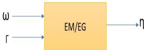
**Figure 3.7:** The figure shows the block diagram of the EM map. The electric machine map is a function of electric machine speed and electric machine torque and returns the efficiency of the corresponding speed and torque.
