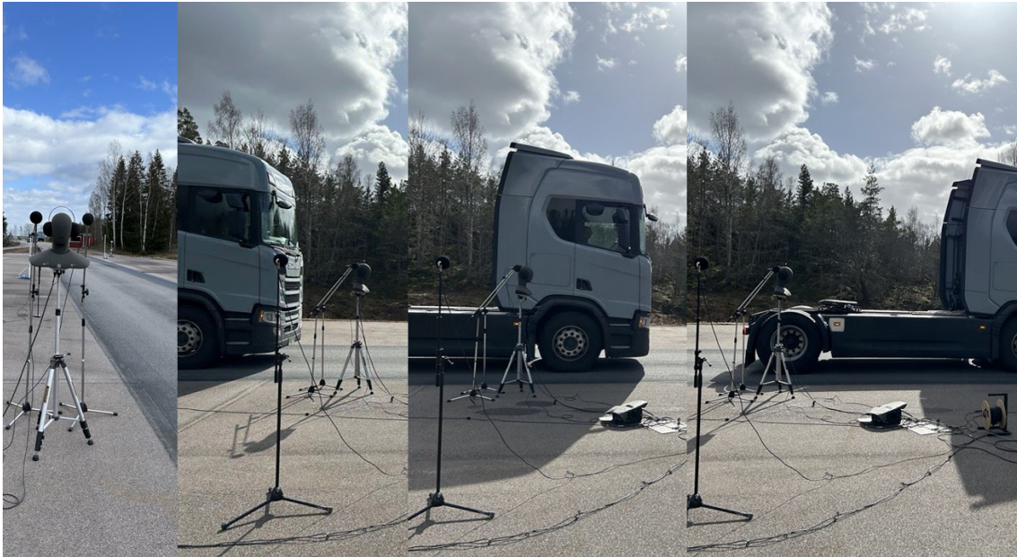
Figure 3.2: Photos Taken During BEV Truck Measurements, Scania Test Track, Södertälje.
