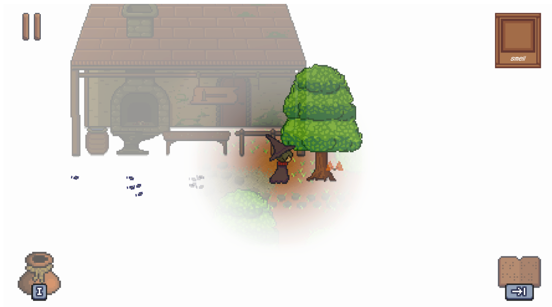
Figure 5.11: Image shows how the large building shows up even though only it being partly in the players field of view. Note that the large building is faded out because of its distance to the player.
