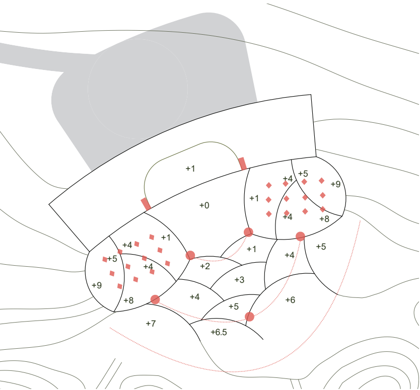
Cross firing clusters (front zone), overhead distribution grid (seated zones), and line array positions (middle and back zones).
