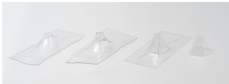
Figure 9.15: Vacuum forming experiments for tip manufacturing.
