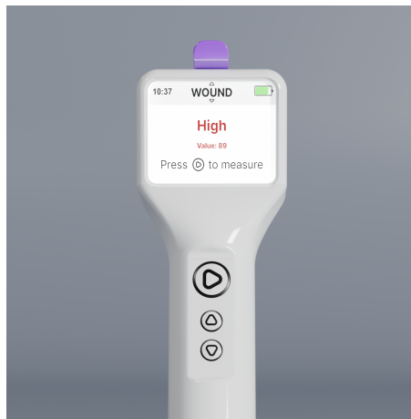
Figure 10.5: Scanner interface, showcasing buttons and screen.
