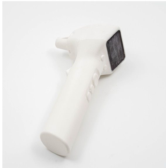
Figure 9.19: Prototype with multiple button layout options.
