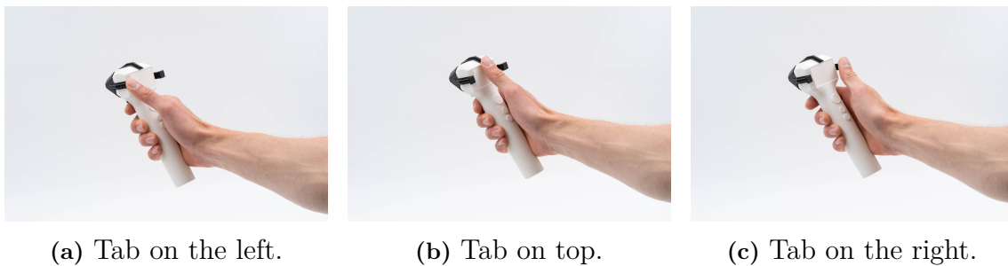
Figure 9.17: Three locations of ejection tab.
