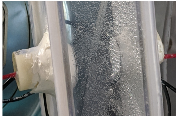
Figure 4.10: Image showing the bubbles on the surfaces of the sensor box and the transducer.
