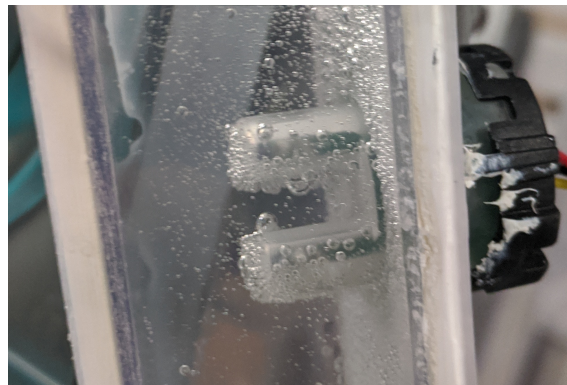
Figure 4.19: Image showing the air bubbles on the surfaces of the sensor box and the turbidity probe.
