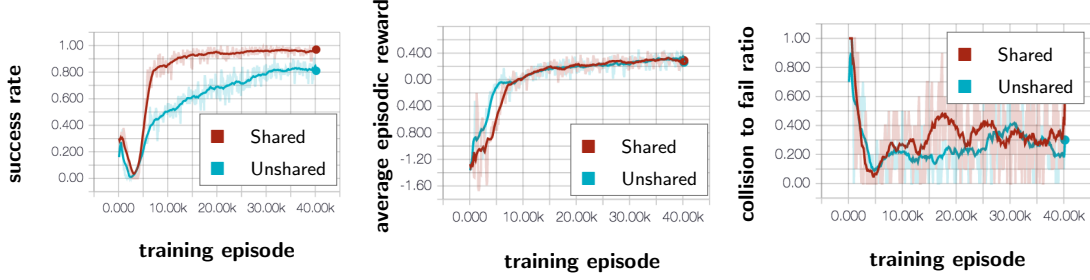
Figure 5.2: The figure shows that the success rate for a network with shared weights (brown line) converge faster than the fully connected network structure which do not share weights (turquoise line).
