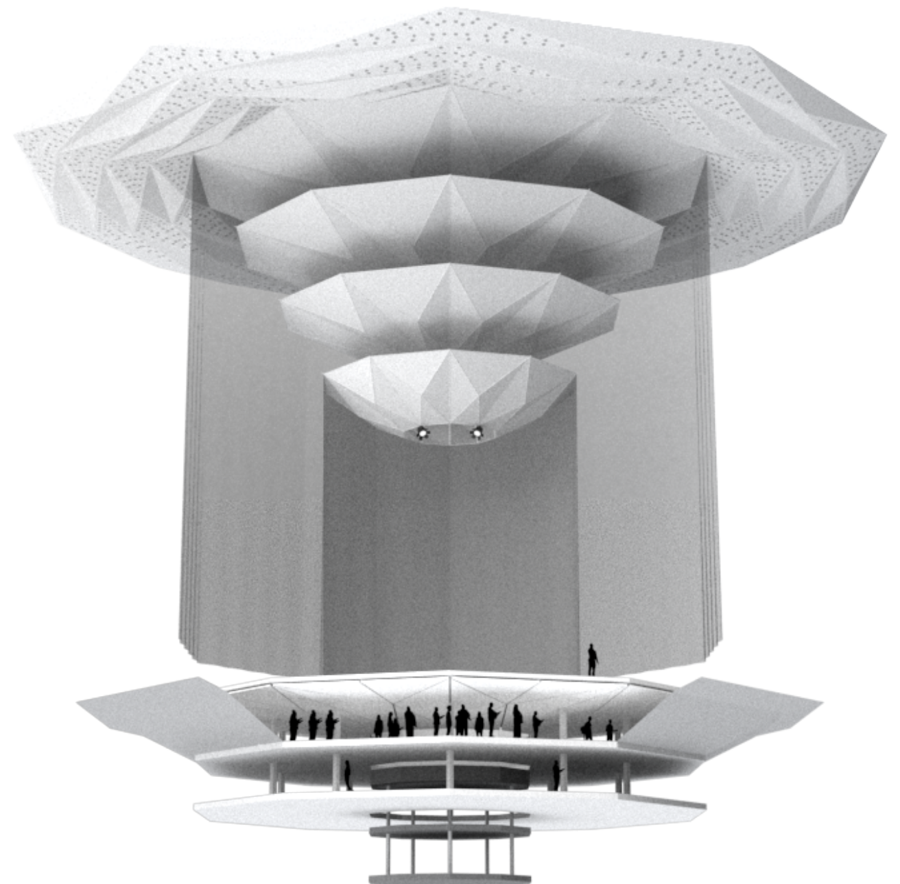
Illustration of the stage and stage reflector prototypes
