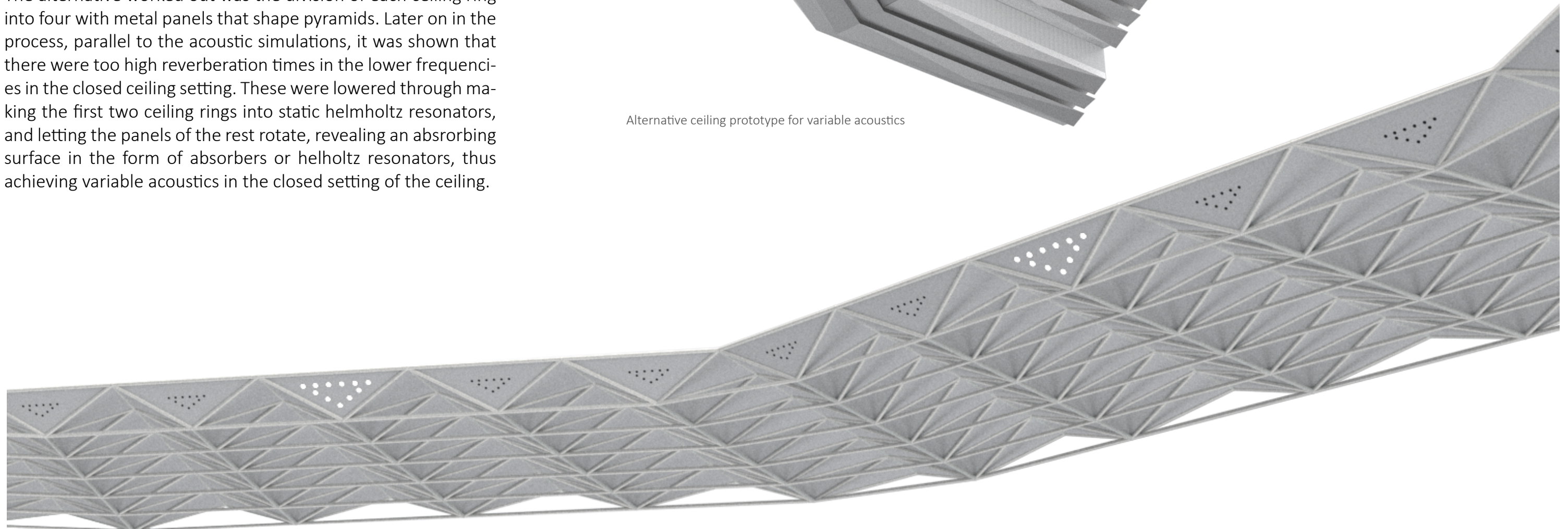
First ceiling prototype for variable acoustics, with a paneling of the truss' pyramids
