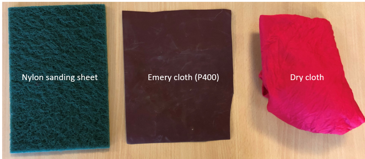
Figure 3.6: Illustration of the objects used for the mechanical surface preparation of the connections.
