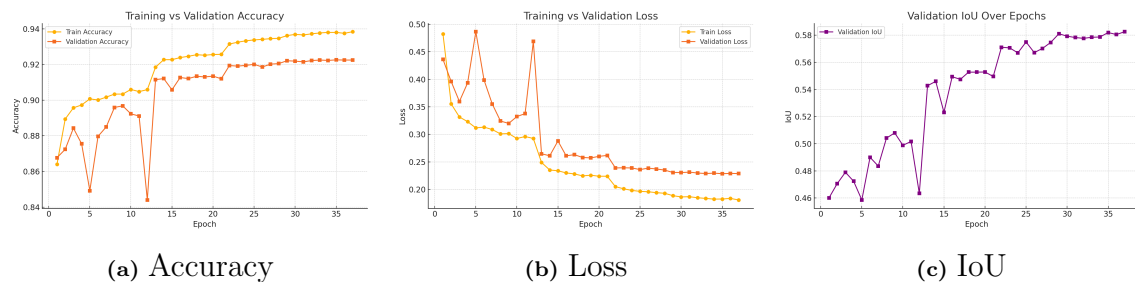
Figure 4.6: Training and validation metrics (accuracy, loss, and IoU) for FCN-ResNet18 over 37 epochs.
