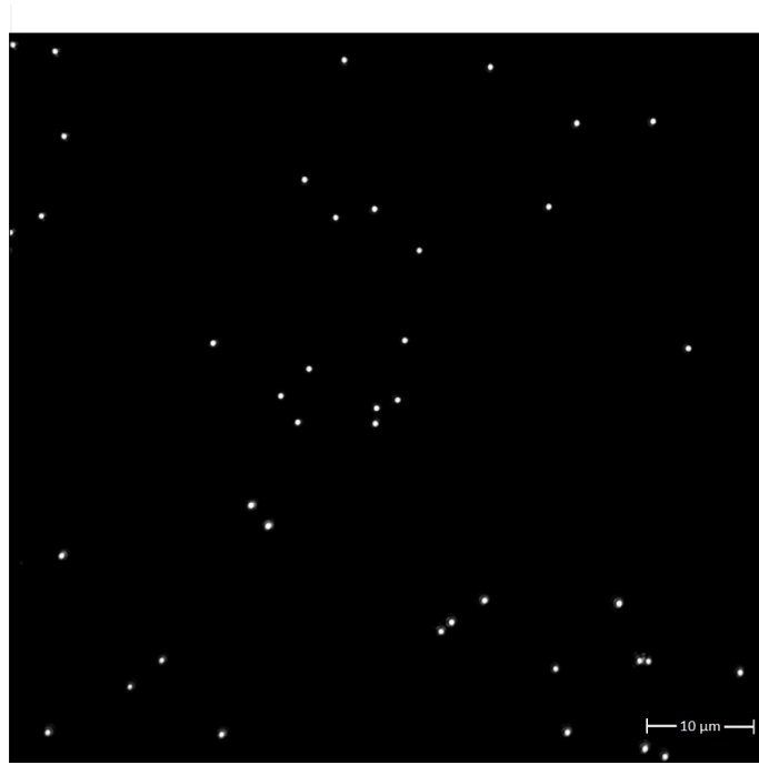
Figure 4.16: Optical image of 100 nm diameter disks consisting of 1 nm Ti and 25 nm Au, illuminated by 635 nm 1750 mV laser light coupled through a waveguide. Note that the bright spots in the image are not the actual disks, as is the case in the SEM images previously shown, but instead laser light scattered from the disks, which themselves have diameters well below the diffraction limit. The spots in the image have approximately the same size as the 635 nm laser wavelength.
