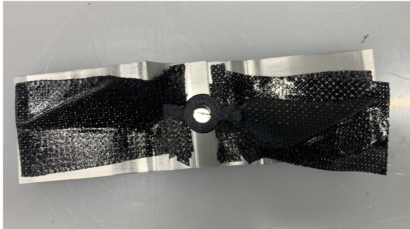
Figure 3.16: Layup of propeller skin – left blade has the bottom skin only, while right blade has the bottom and middle layers.
