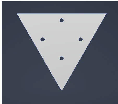
Figure 3.10: Sketch of the motor attachment/front bulkhead in CAD.
