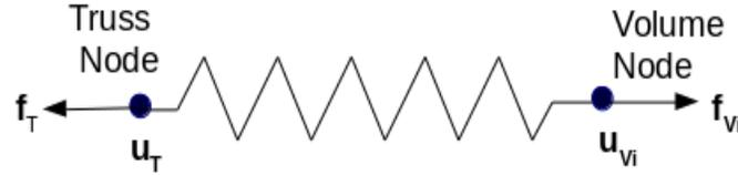
Figure 3.11: Imaginary spring connecting the truss node and the volume node.
