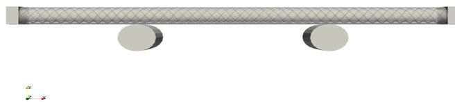
Figure 3.17: Three point bending FE model.
