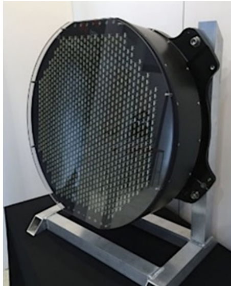
Figure 2.1: An AESA antenna
