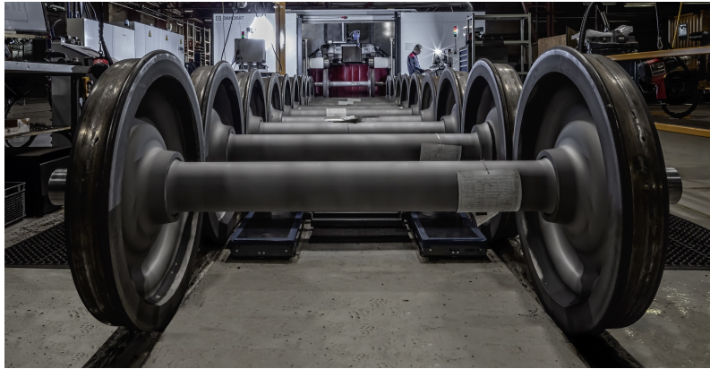
Figure 2.2: Wheelsets stored for maintenance
