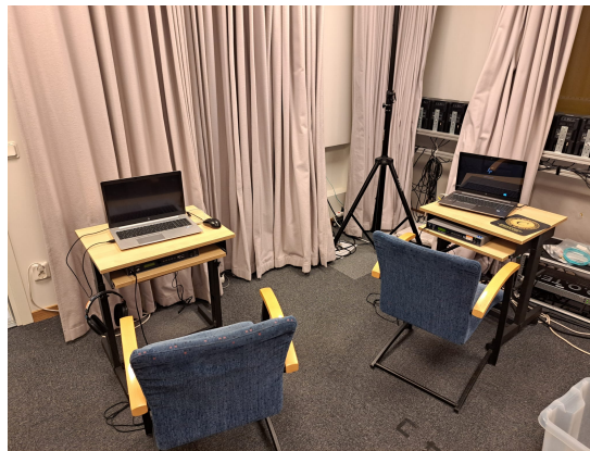
Figure 3.11: Listening test setup at Chalmers: simplified environment without car seats.
