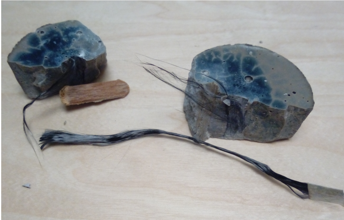
Figure 22: Experiment 4 after pullout
