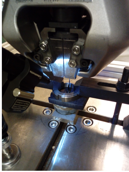
Figure 12: The set up used to test the pullout strength of samples
