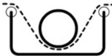
Figure 7: Impregnation of a fibre bundle using an open bath[37]
