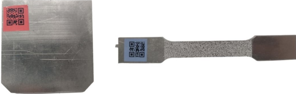
Figure A.2: Aluminium test sample for bending (left) and tensile(right).
