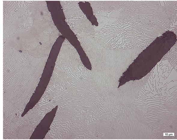
(b) In 500X magnification, the lamellae structure of the pearlite is visible.
