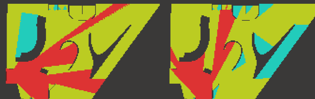
Figure 4.8 The visual step depth from each entrance. The red area shows what is visible from the entrances. The yellow area shows what is visible from the red area. The blue area shows what is visible from the yellow area. In other words, from red to blue you reach deeper in the space.
