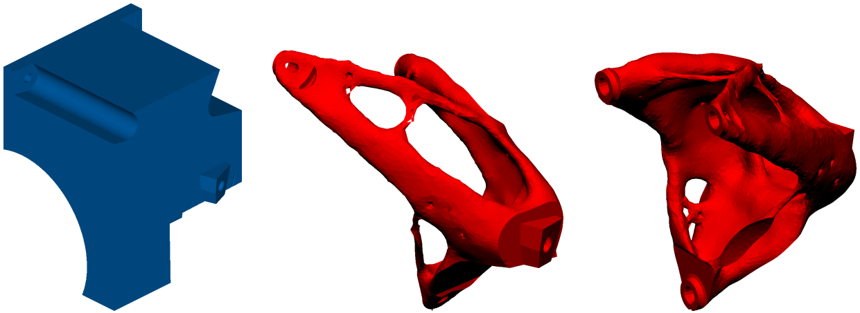
Figure 4.6: Optimal stiff material distribution inside the design space (100% m_0 , no demoulding direction)
