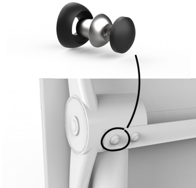
Figure 68: Collision protection on the cable tray
