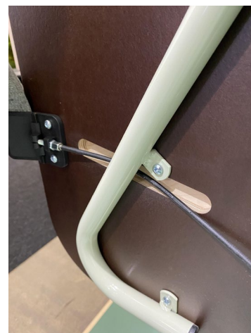
A cut out made for easier cable management
