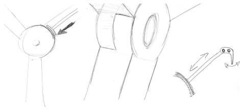
Figure 26: Shows a friction and clamp inspired lock
