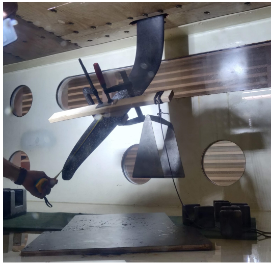
(a) Placement of test load at leading edge
