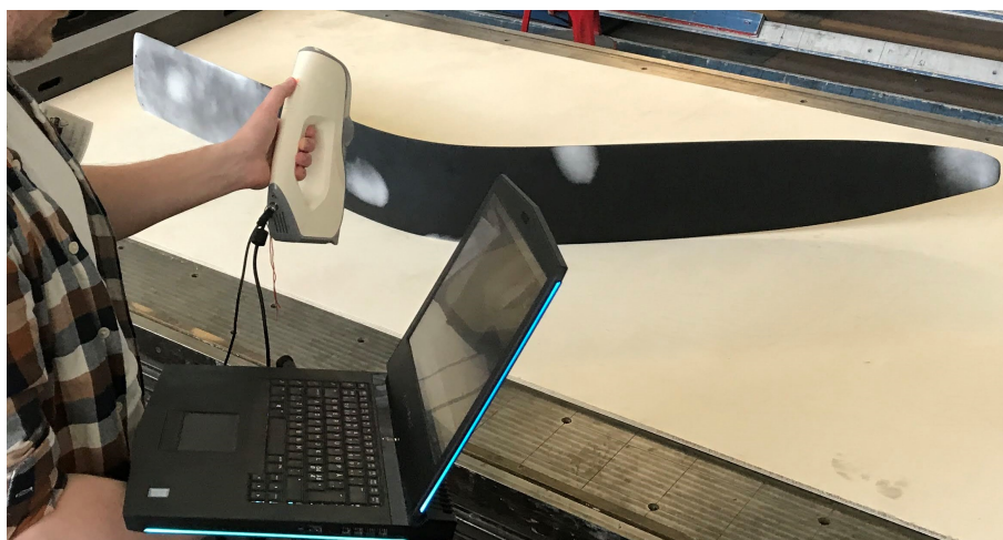
Figure 4.8: Attempted scanning of the partly painted foil
