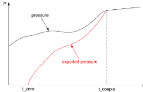
Figure E.1: Pressure Ramping methodology scheme Siemens, 2020
