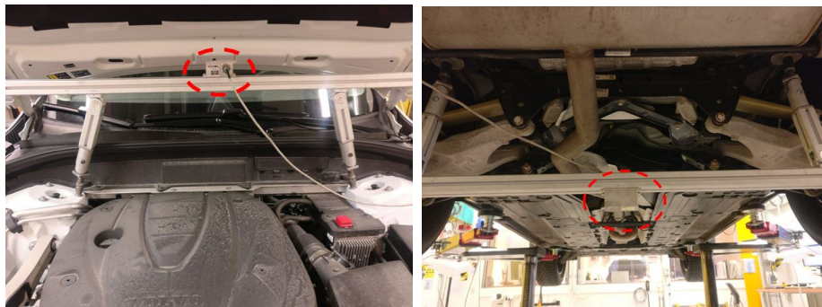
(a) Front: Between the strut towers (b) Rear: Between sub frame attachments
