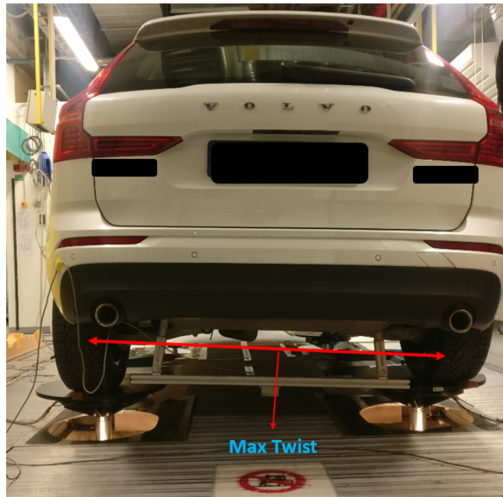
Figure 4.17: Maximum twist in the Model B for the test-rig experiment
