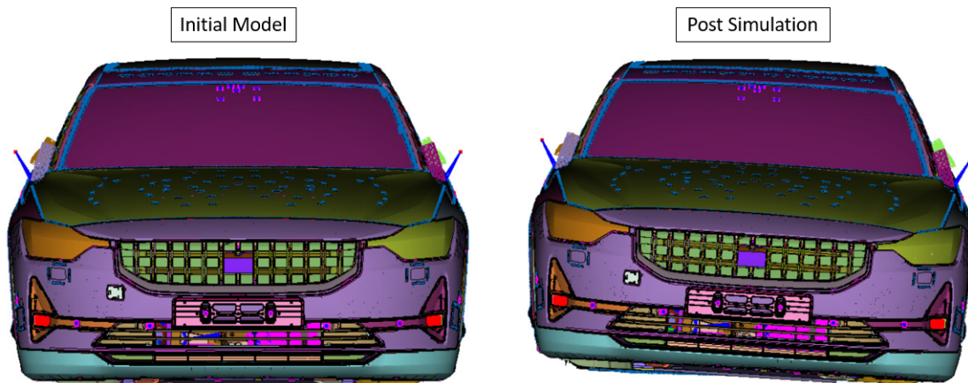
Figure 4.8: Post-processed result for the wheel load from Meta - Front view
