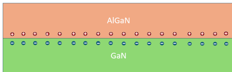
Figure 2.14: Polarization AlGaN and GaN interface.
