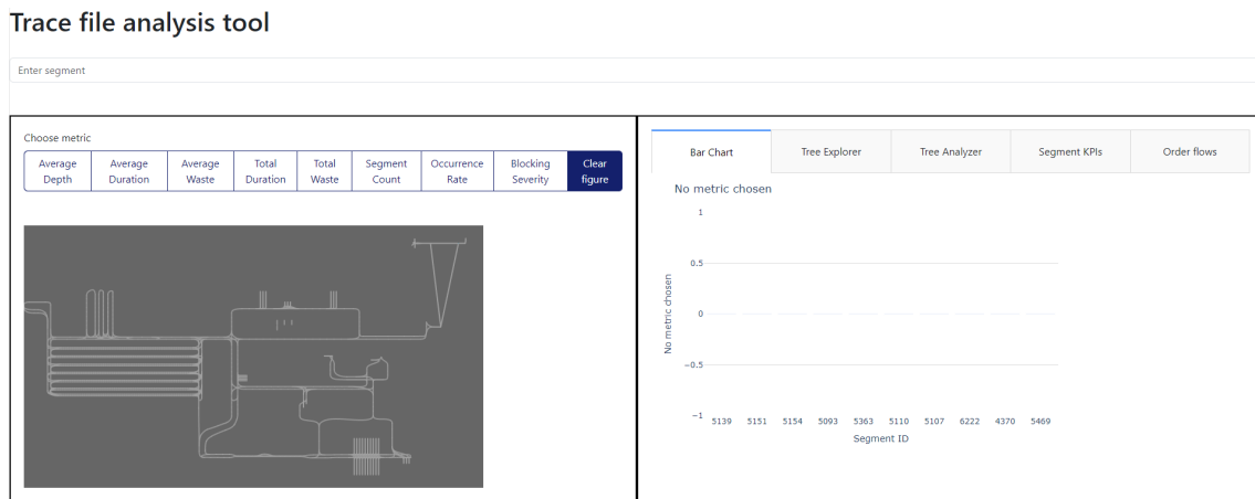
Figure 5.1: Startup view of the visualization tool. On the left the user is presented with a physical view of the entire layout and a set of different metrics to display. Since no metric is chosen the bar chart on the right is empty.
