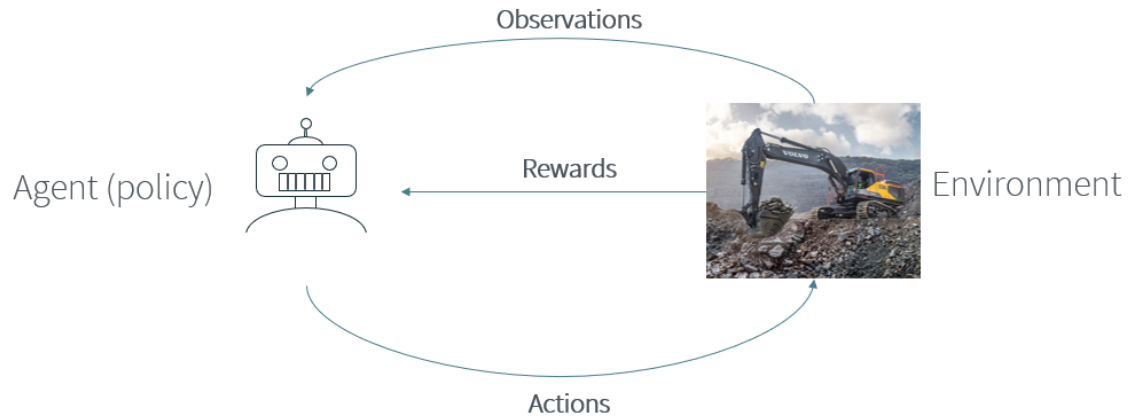
Figure 2.5: Visualization of RL system. The agent takes actions based on the observations and rewards calculated from the environment.
