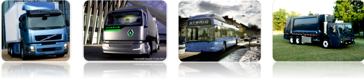
Figure 2.4 Different Volvo vehicles with a diesel electric hybrid driveline. From left to right: Volvo FE Medium Duty distribution vehicle , Renault Premium Distribution Hybrys , Volvo 7700 hybrid city bus and MACK® TerraPro™ Low Entry refuse truck (The Volvo Group, 2009).
