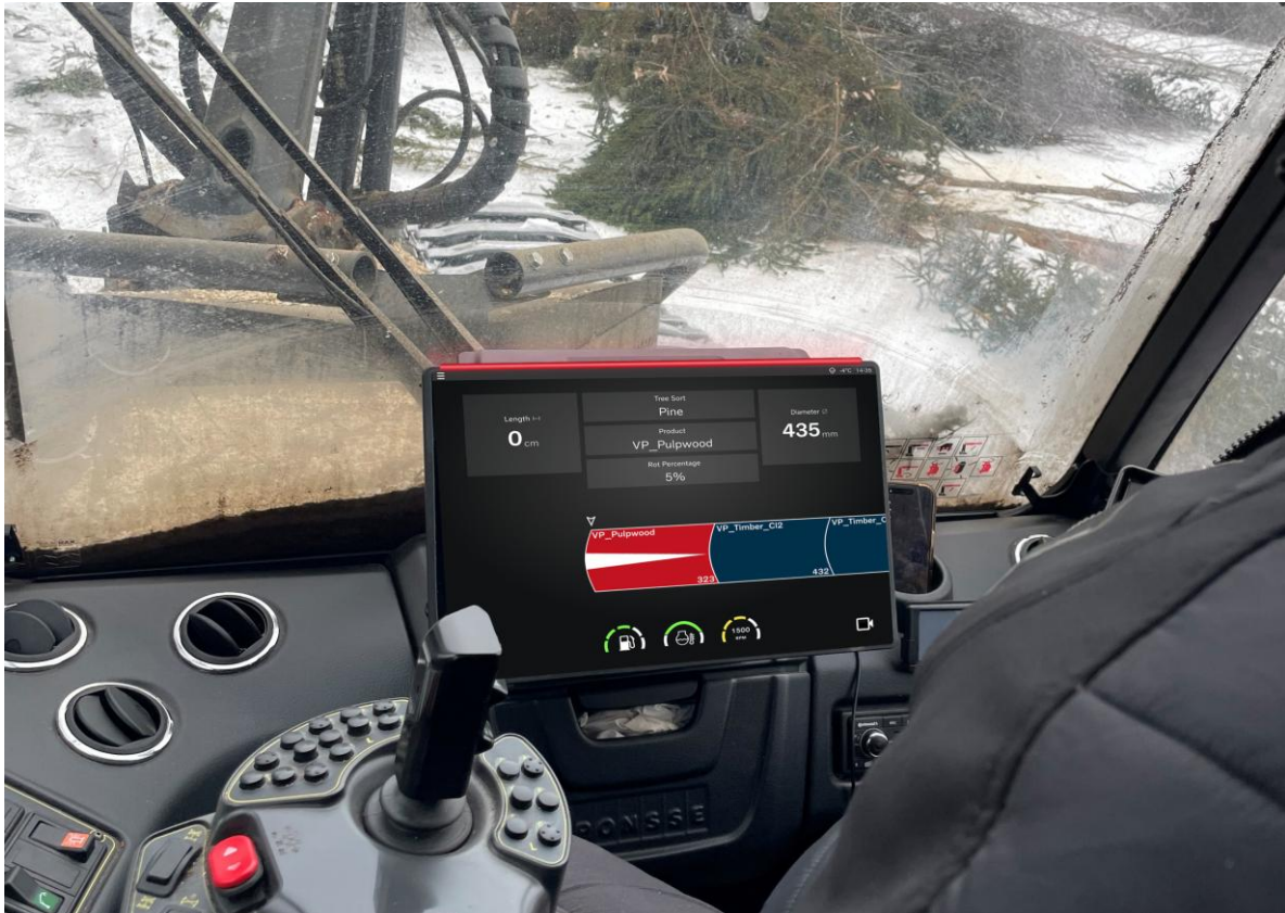
Figure 62. LED light to detect rot that is placed on top of the main display in the harvester.
