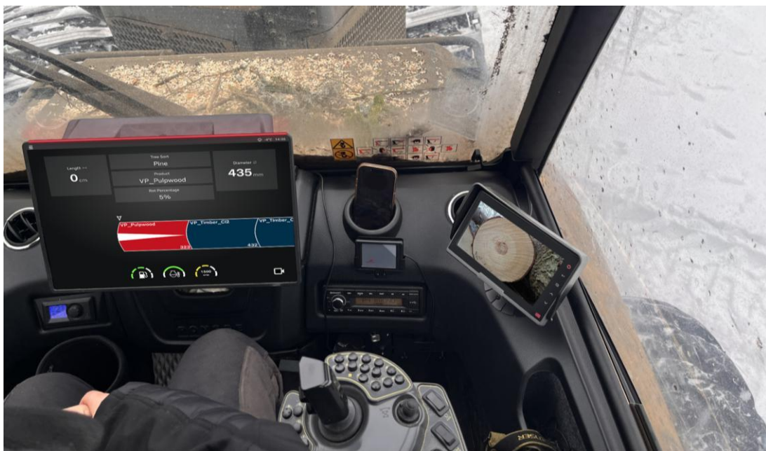
Figure 1. Final design in context of a harvester cockpit. The design includes a bucking assistance interface, a LED-light for detection and a cross-section view of the cut log.
