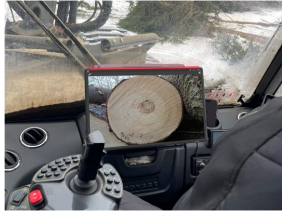
Figure 4. The cross-section view in the harvester:
