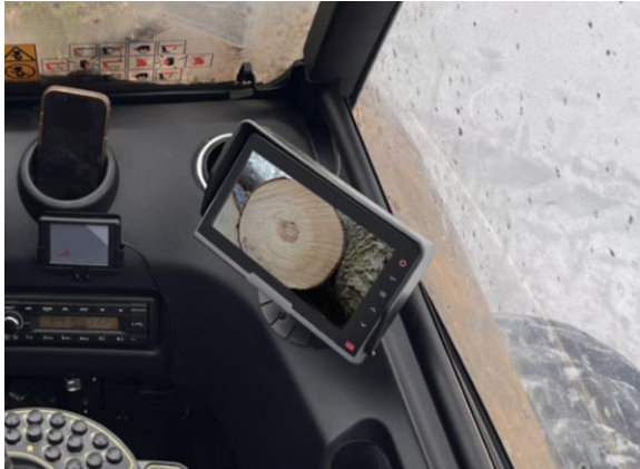
Figure 4. The cross-section view in the harvester:
