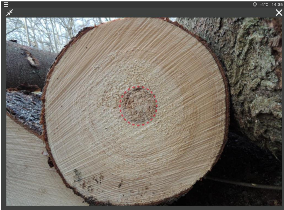
Figure 58. Full screen cross-section view on the main display. The red circle marks the rotten part of the log.
