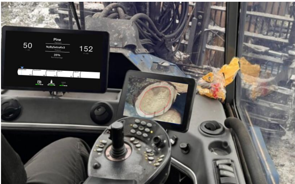
Figure 47. Placements of the refined cross-section concept, where it is placed on the reversing camera display.
