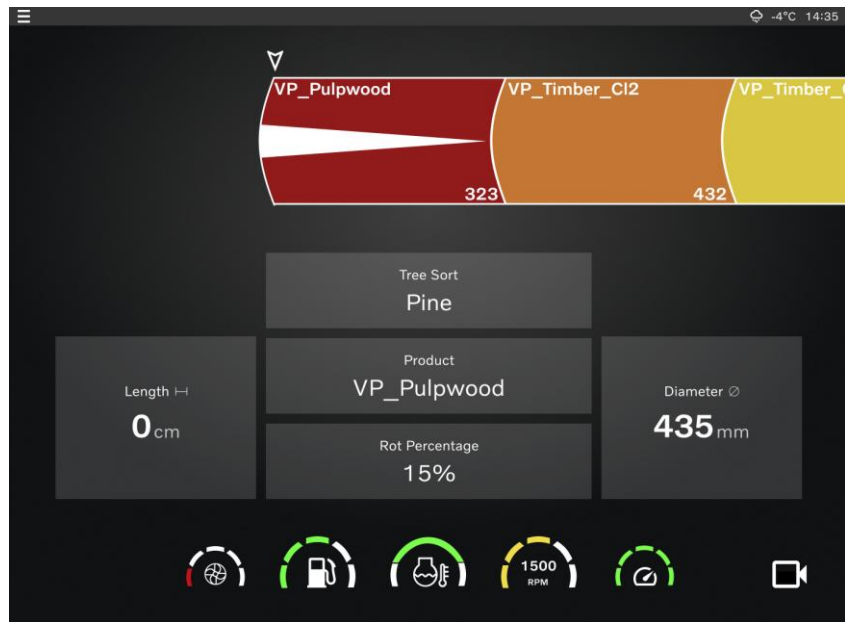
Figure 6. Customized bucking interface illustrating modified layout, log color scheme, and a change of taskbar icons.
