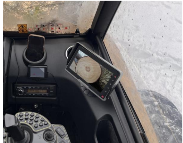
Figure 59. Full screen cross-section view: a) on main display b) on reversing camera display
