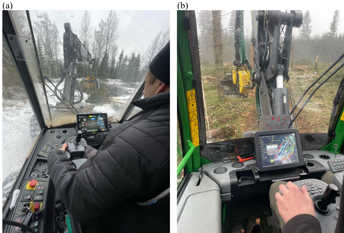
Figure 10. Examples of joysticks and keyboards in different harvesters used in forestry operations:
