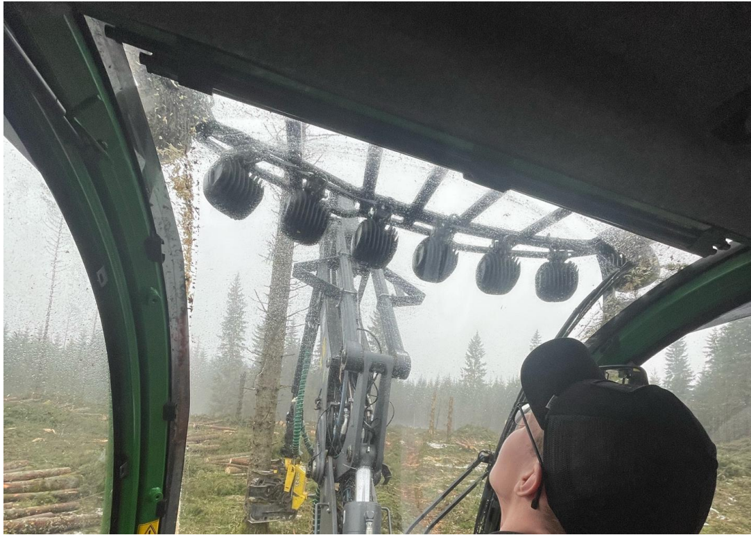
Figure 9. Lights positioned on the roof of the harvester.
