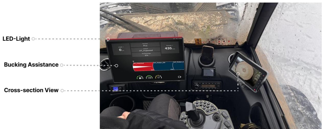
Figure 52. Final design in context of a harvester cockpit. It includes the features of a bucking assistance interface, a LED light for detection of rot and a cross-section view.
