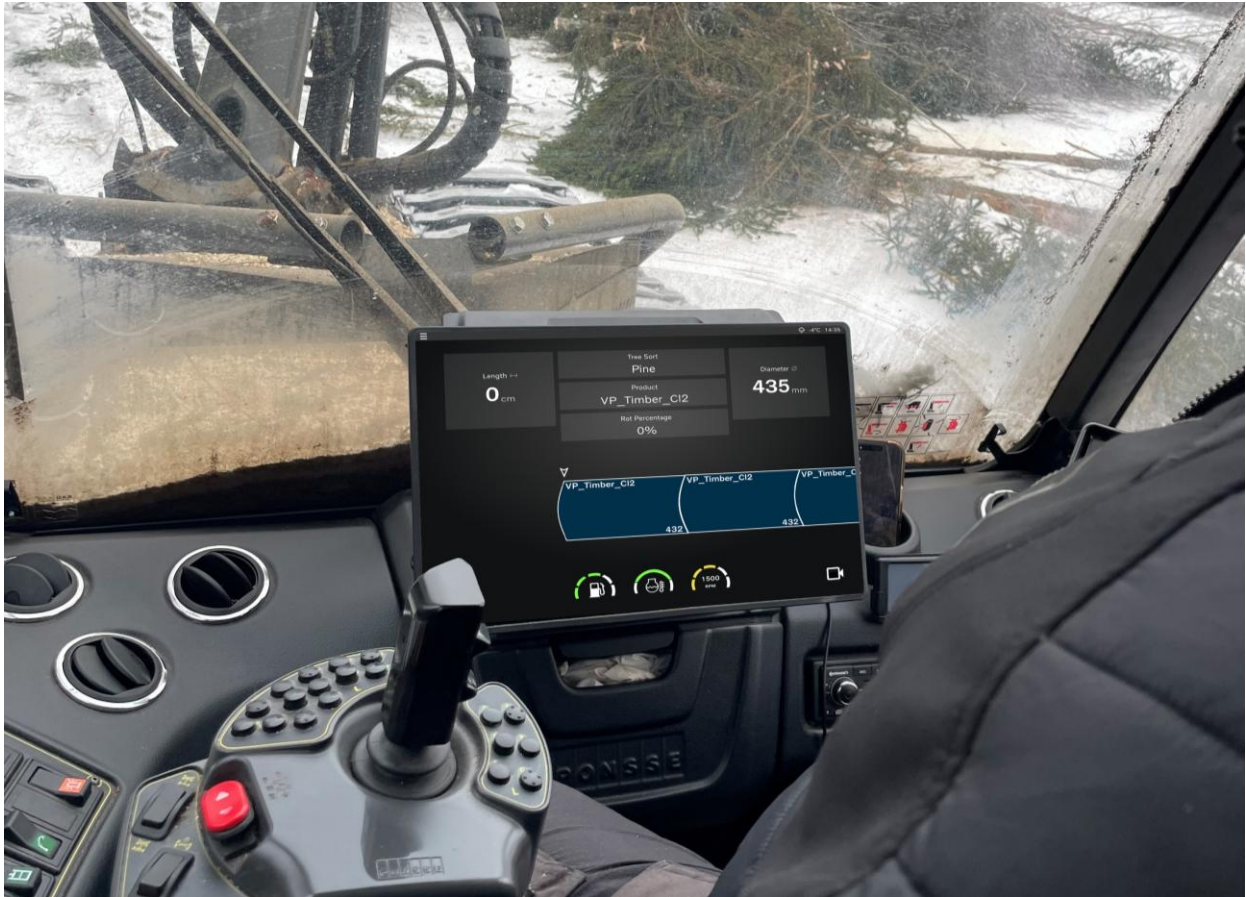
Figure 53. The final design interface when bucking a normal tree. The logs are blue and no rot is visible on the screen.
