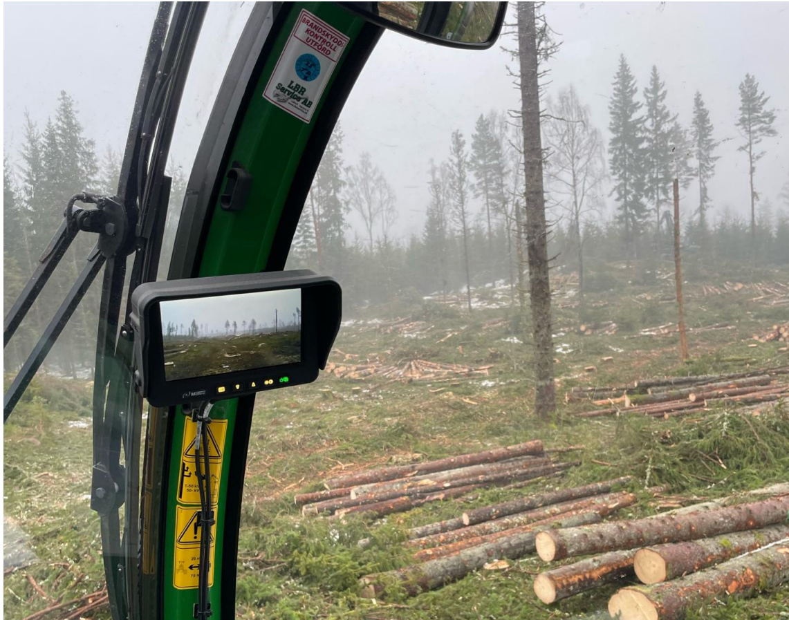
Figure 12. Reversing camera view and placement in a John Deere harvester.
