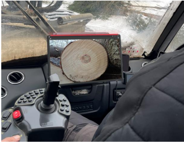
Figure 59. Full screen cross-section view: a) on main display b) on reversing camera display
