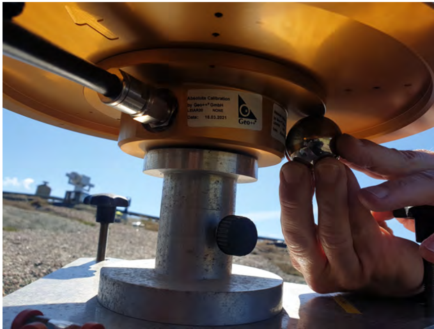
Figure 3.3: Small object of the tracker measurement on antenna
