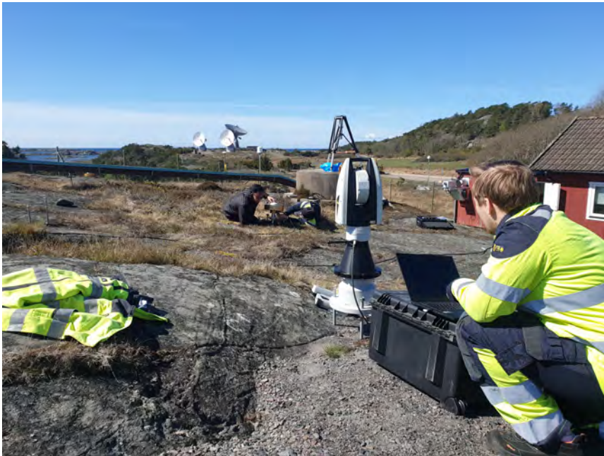
Figure 3.2: Laser tracker measurement
